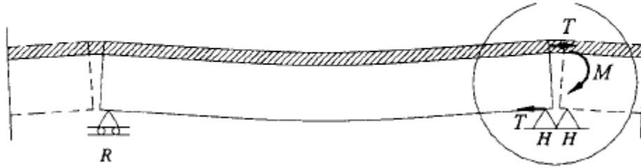
Figure C-3. Effect of RHHR type support condition on continuity (Okeil and El-Safty 2005)
