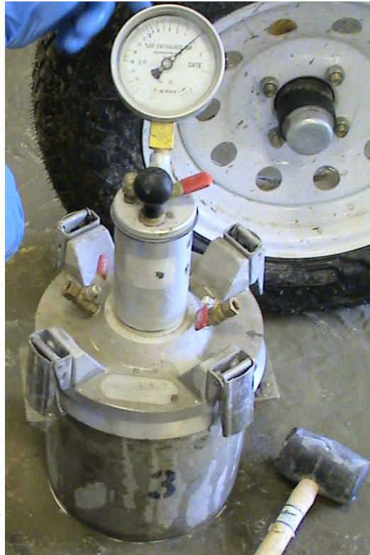
Figure 3-33. Determination of air content.
