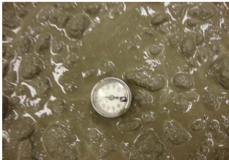
Figure 3-34. Determination of temperature of mixture.
