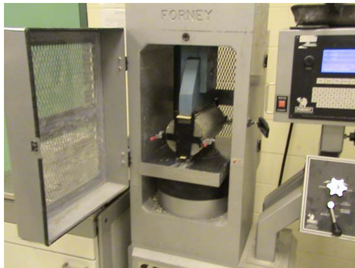
Figure 3-41. Splitting tensile setup.
