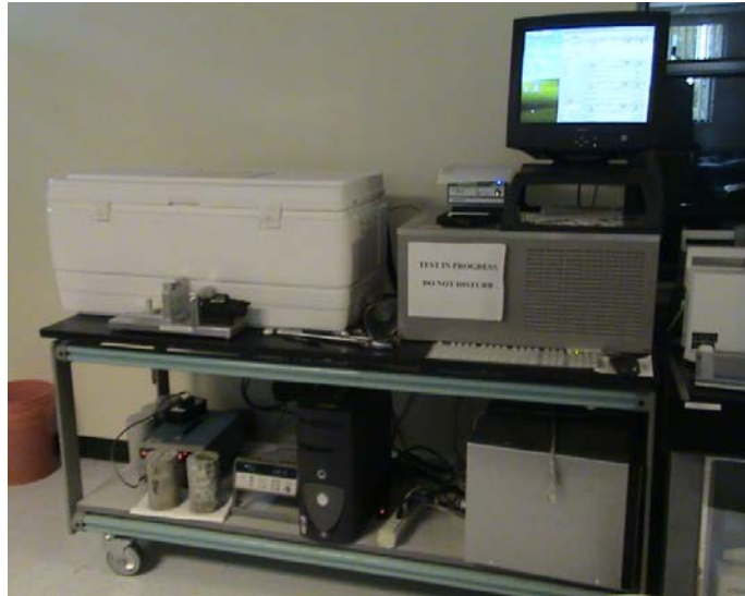
Figure 3-44. Coefficient of thermal expansion setup.
