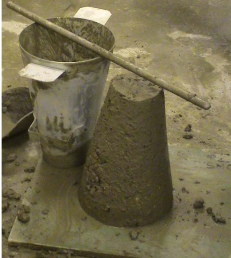
Figure 3-31. Determination of slump.
