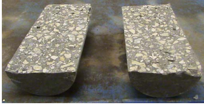
Figure 3-42. Failed sample from splitting tensile test.
