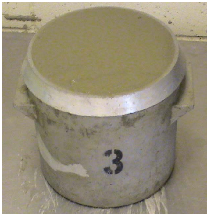
Figure 3-32. Determination of unit weight.
