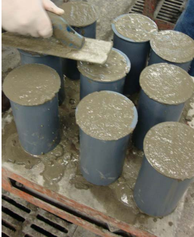
Figure 3-28. Cylinders on vibrating table.
