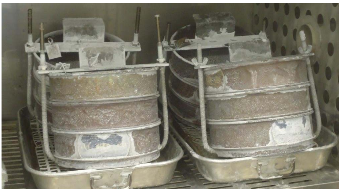
Figure 3-21. Sodium sulfate samples in oven.
