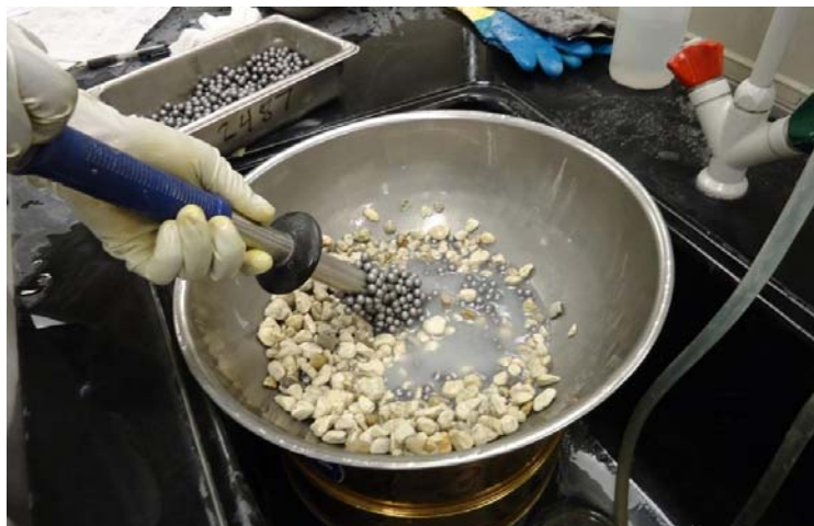
Figure 3-18. Steel balls being removed from aggregate after Micro-Deval test.
