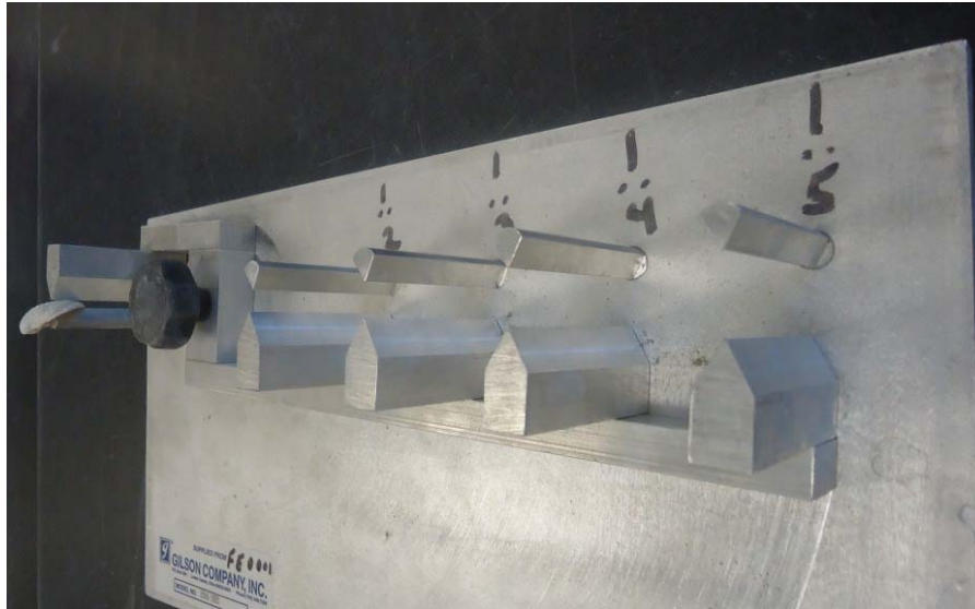
Figure 3-23. Caliper for determining free shell content.
