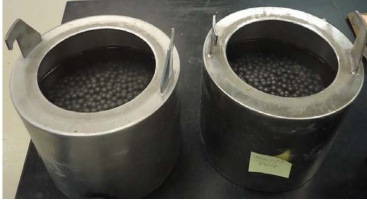
Figure 3-16. Soaked aggregate with steel balls before Micro-Deval test.
