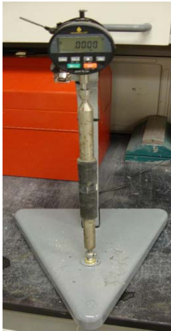
Figure 3-43. Free shrinkage setup.
