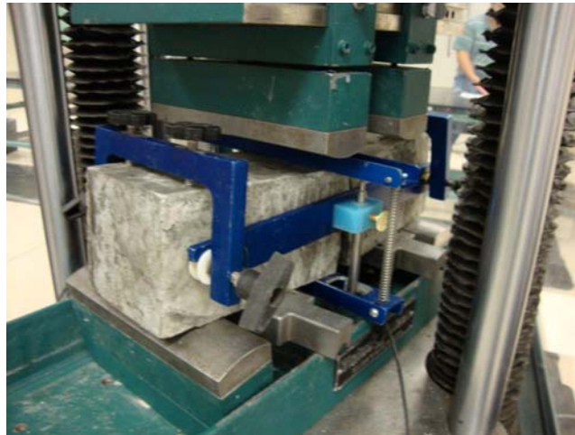
Figure 3-39. Flexural test setup.
