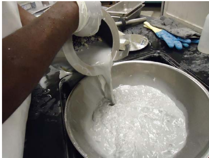
Figure 3-17. Aggregate being poured after Micro-Deval test.
