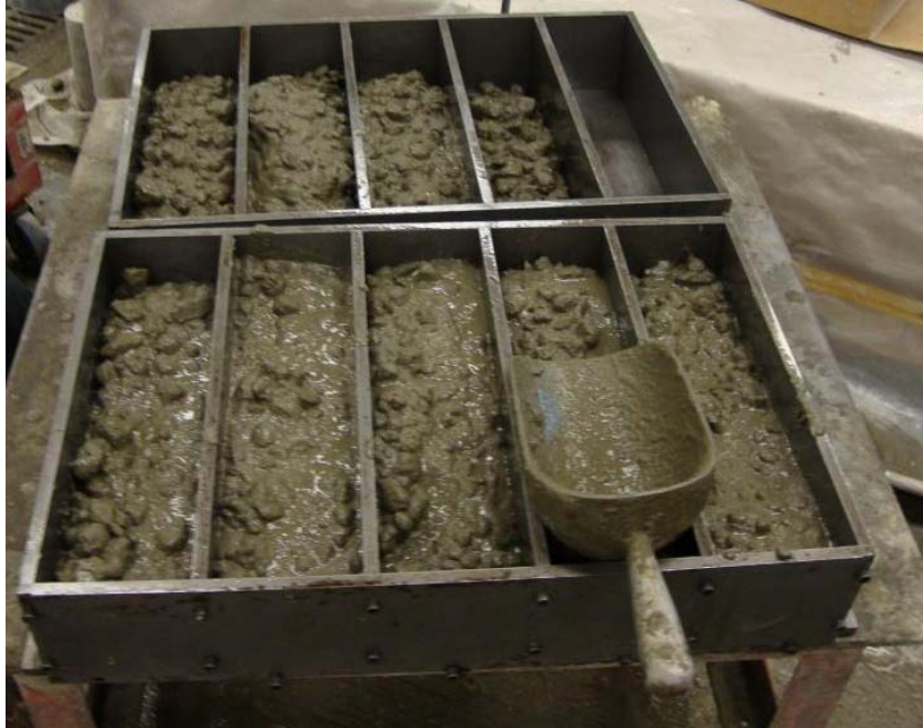
Figure 3-30. Beams on vibrating table.
