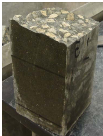
Figure 3-40. Failure of sample under flexural test.
