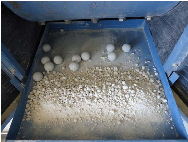
Figure 3-13. Aggregate and steel spheres after Los Angeles abrasion loss test.
