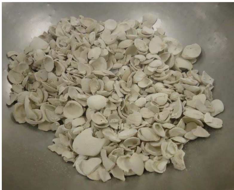
Figure 3-24. Free shell removed from aggregates.
