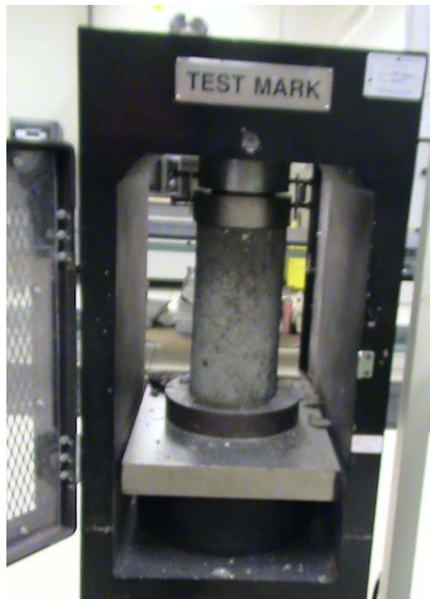
Figure 3-37. Sample in compressive test.
