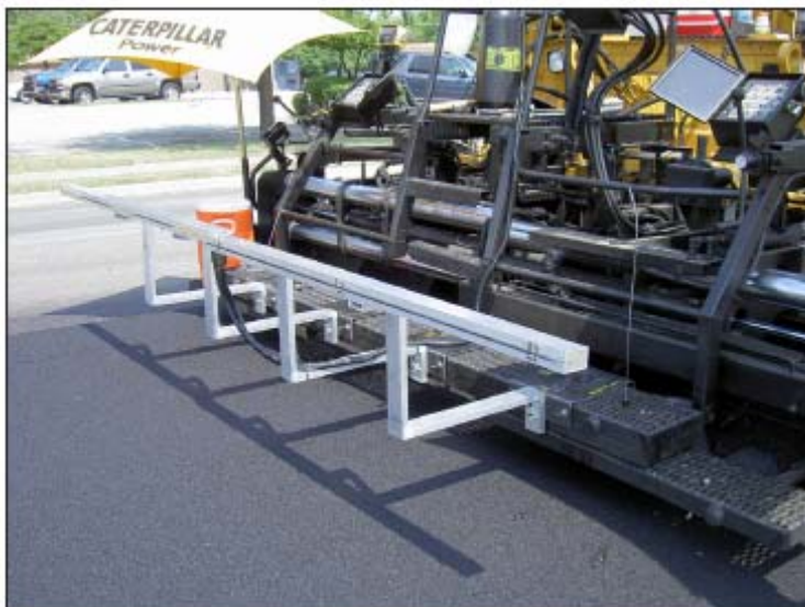
Figure 1-7. The Infrared System Installed on a Paver (Scullion et al. 2006).
