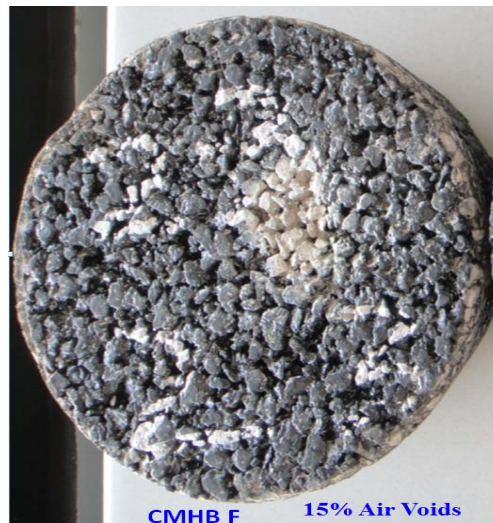
Figure 5-19. Typical Core from US 87.
