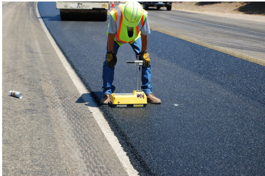
Figure 5-2. Density Measurement on US 87 in the Austin District.
