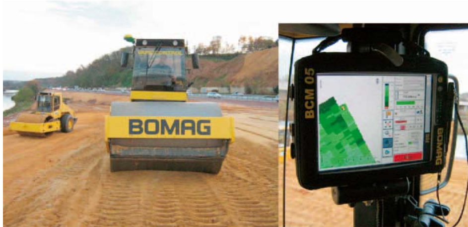
Figure 1-19. Components of the Bomag IC Software (Kloubert et al. 2007).
