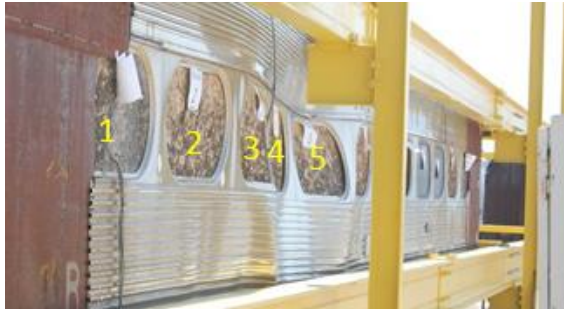
Figure 5. Deformation of Car 244
