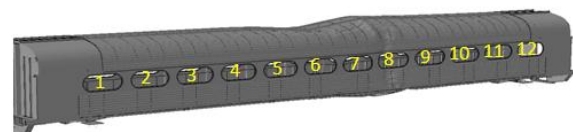
Figure 3. Predicted Carbody Deformation
