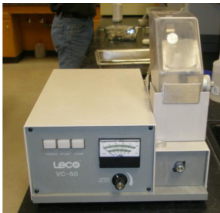
FIGURE 2.1 Leco VC-50 Precision Saw Used to Remove Limestone Aggregates from Concrete Cores
