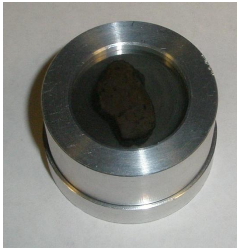
FIGURE 2.4 Polished Aggregate Sample in Custom-Made Aluminum SEM Sample Mount
