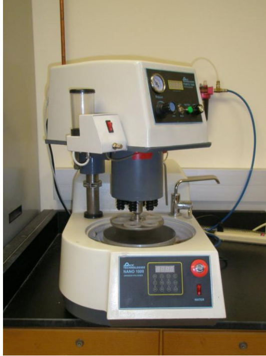
FIGURE 2.2 NANO 1000 Grinder Polisher with FEMTO 1000 Automated Polishing Head Used in this Study
