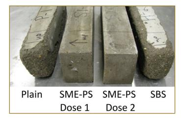
Freeze-Thaw samples after 280 cycles. Untreated (plain) samples and SBS treated samples show significant cover loss. SME-PS treated samples show no visual damage.
