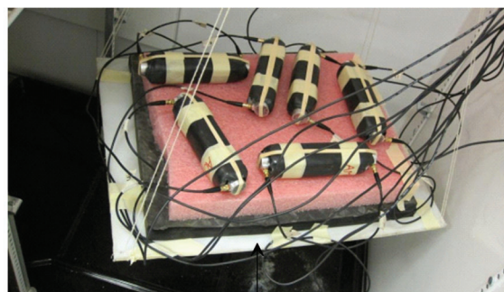
Suspended plate to eliminate vibration and noise from environment
