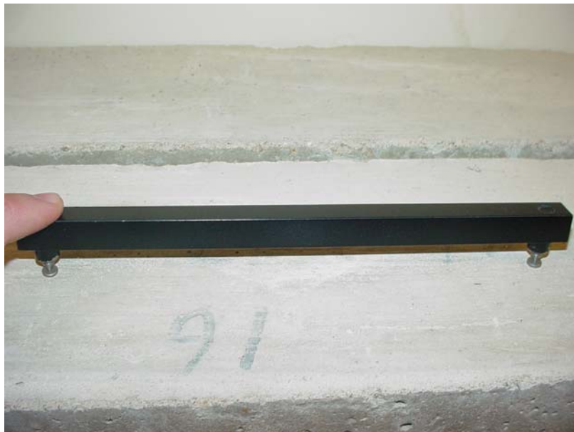
Fig. 3.14: Placing of Measurement Disks with Reference Bar
