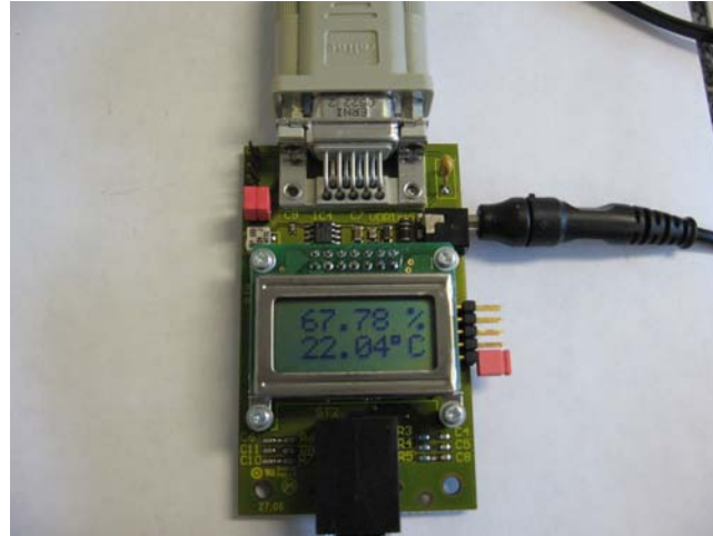
(a) EK-H2 Logger Reads Out Only One SHT75 Temperature and Humidity Sensor
