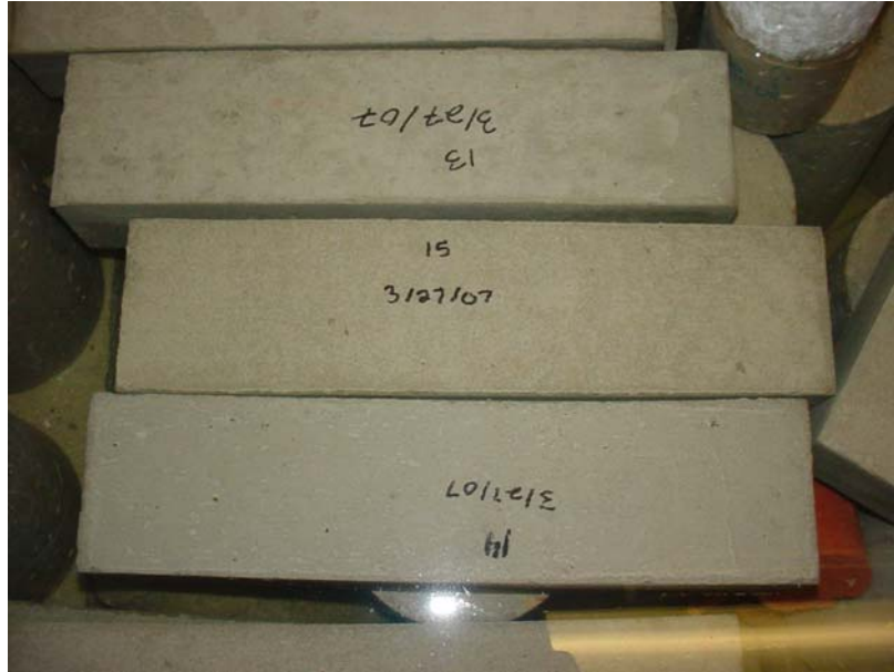
Fig. 3.13: Danish Test Specimens Curing in Water Bath
