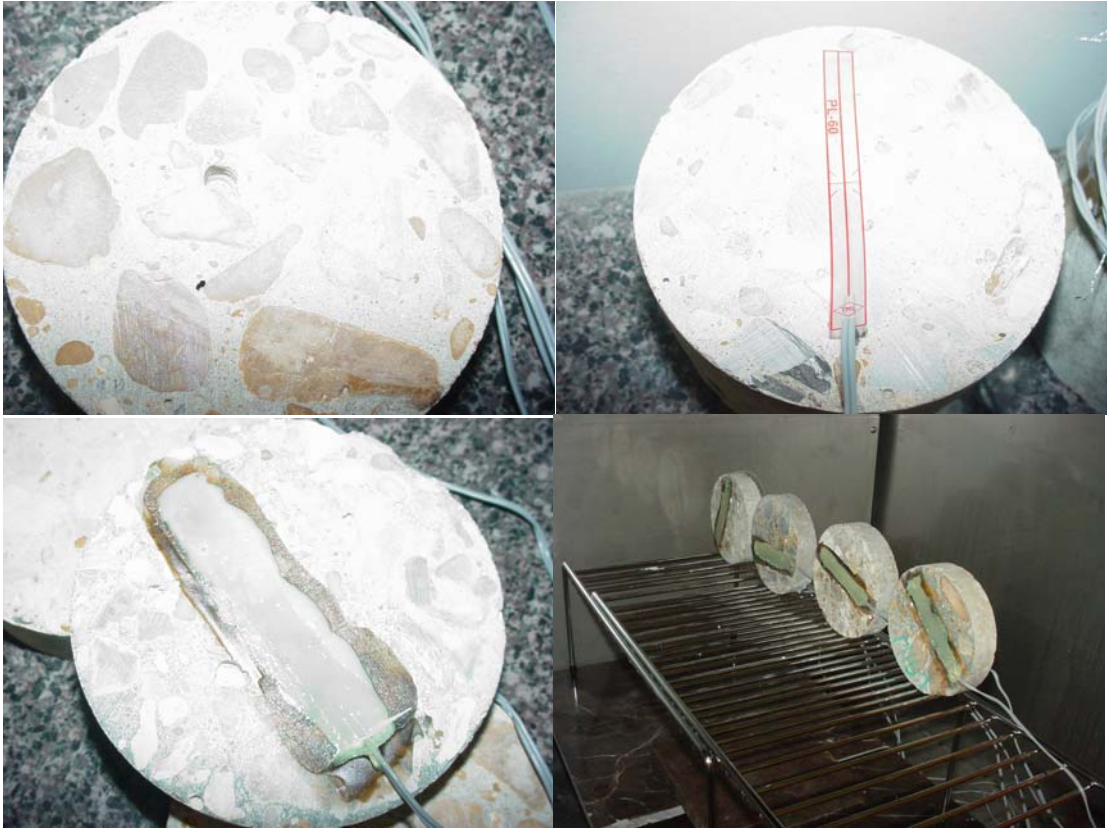
Fig. 3.5: Process of Strain Gage Placement and Measurement
