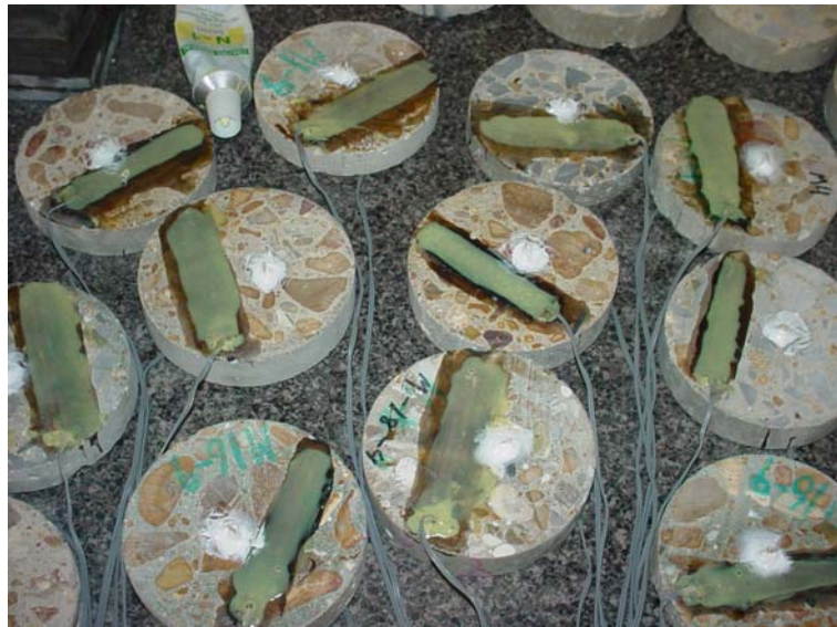
Fig. 3.7: SHT71 Sensor Under Silicone Coating After Placement
