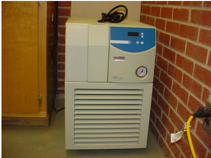
Fig. 3.17: Merlin M75 Chiller Water Temperature Control Unit
