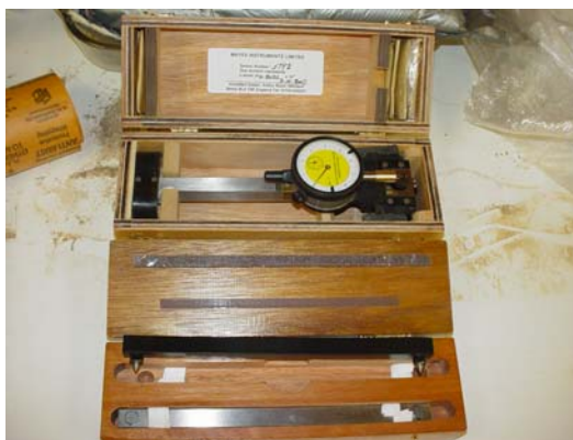
Fig. 3.11: Demec Gauge, Reference Bar, and Calibration Bar
