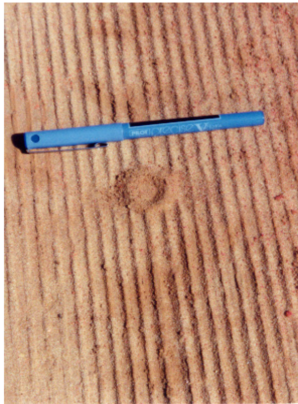
Figure 5.1 Photograph of Imprint Showing Loose Coarse Particles Congregating Around the First Sensor Tip
