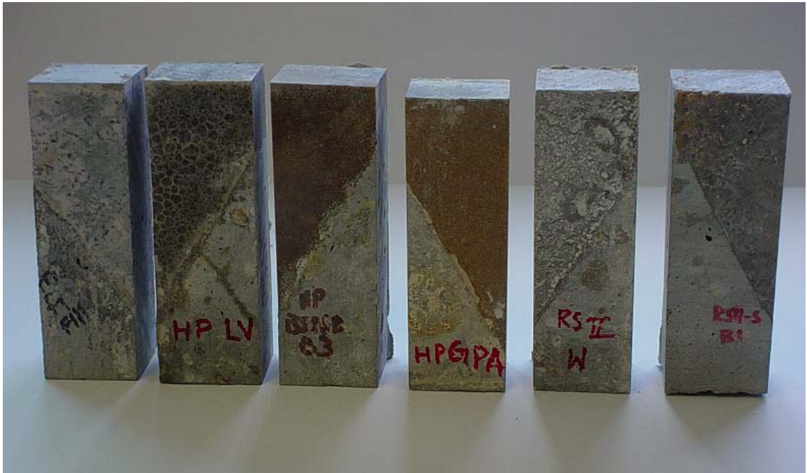
Figure 5.7 Typical test specimen from resin based repair materials (Pot Fill, HP LV, HP Binder, HP GPA, Resurf II Summer, and Resurf II Winter).
