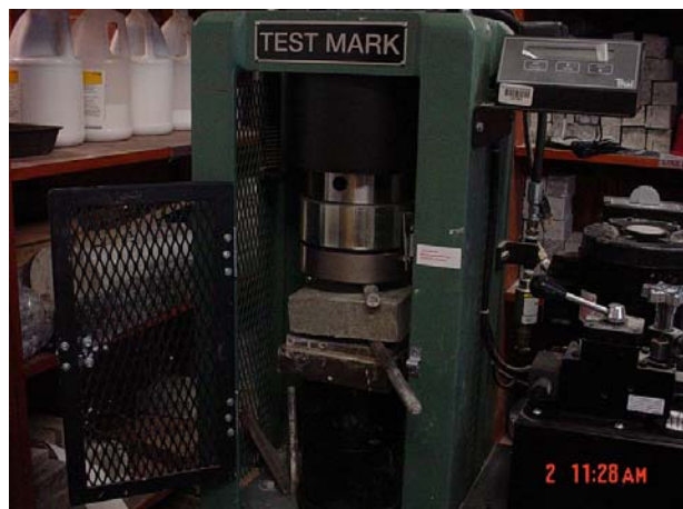
Figure 5.2 Concrete Compression machine was used to split concrete plaques.
