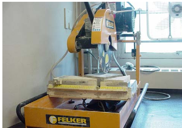
Figure 5.1 A groove was made on every concrete plaque at an angle of 30 degrees.
