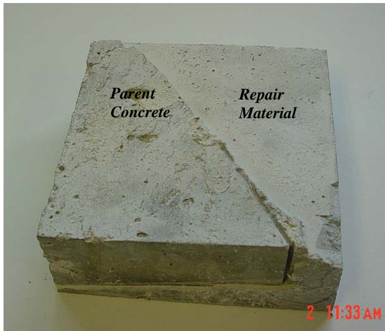
Figure 5.5 Typical repaired concrete plaque.
