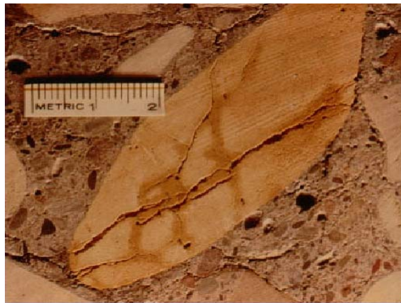
Figure 3.2.15. Aggregate expansion due to alkali-silica reaction [93].
