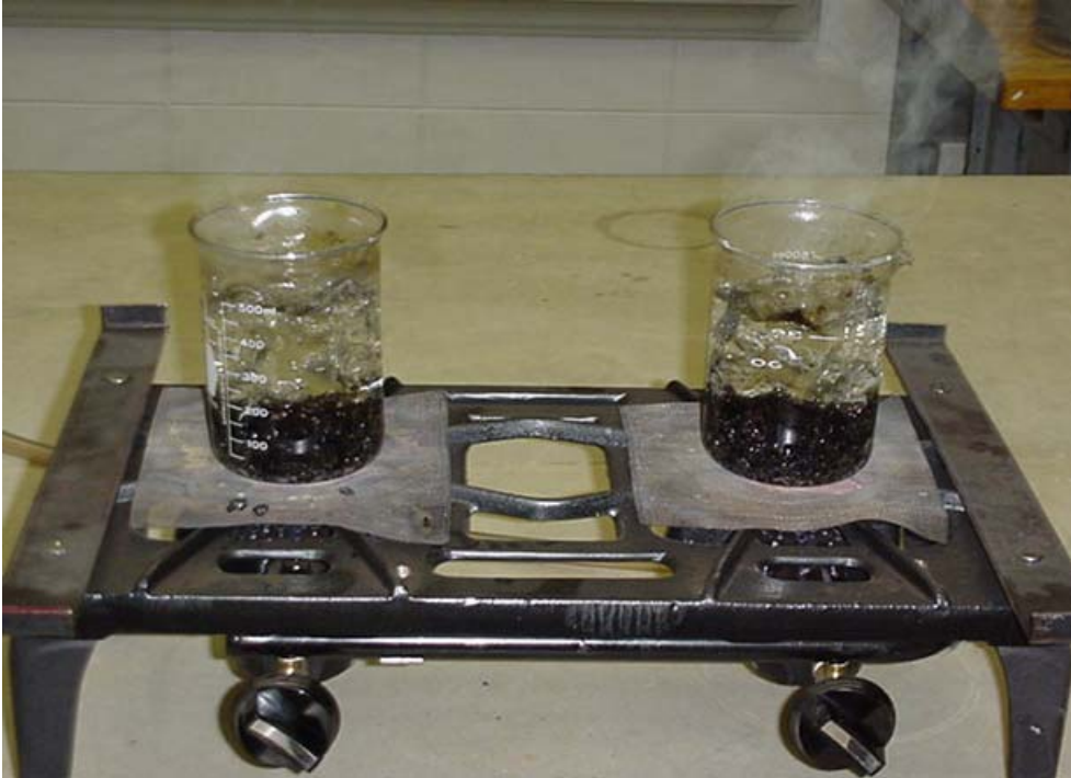
Figure 3.12 HMA Boil Test
