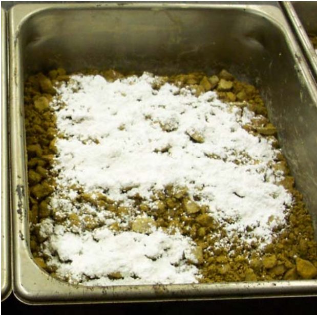
Figure 3.9 Addition of Hydrated Lime
