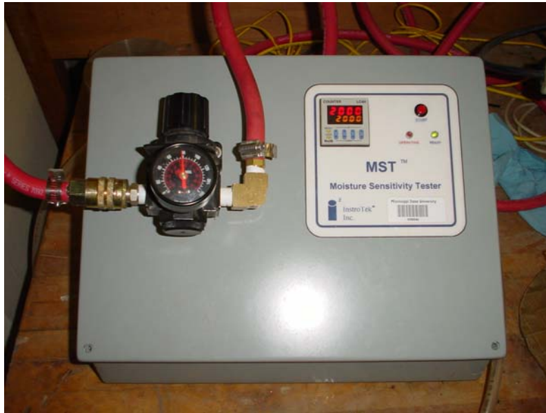
Figure 3.18 Control Unit with Pressure Regulator and Timer
