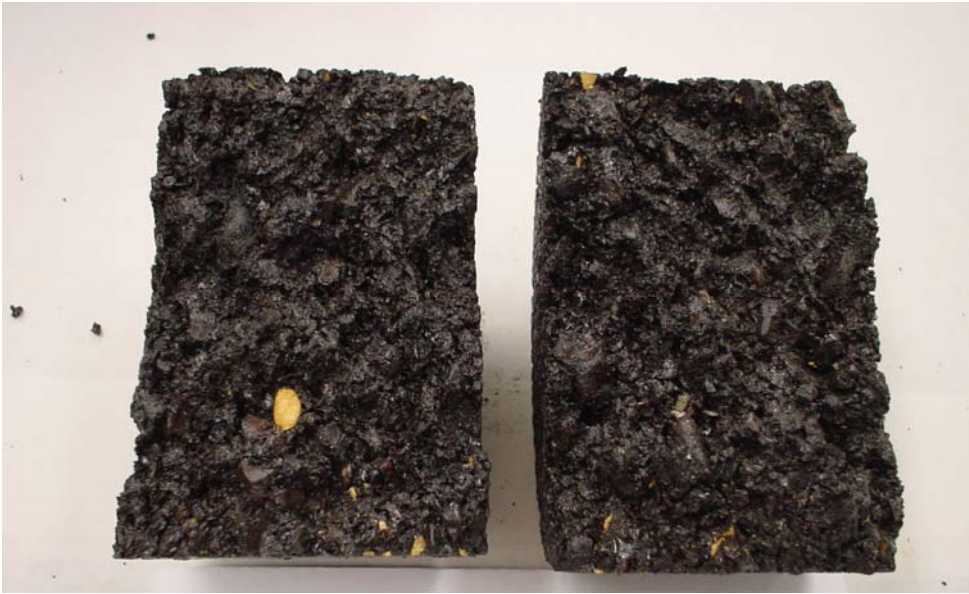
Figure 3.11 Visual Stripping Evaluation of HMA Specimen After Testing
