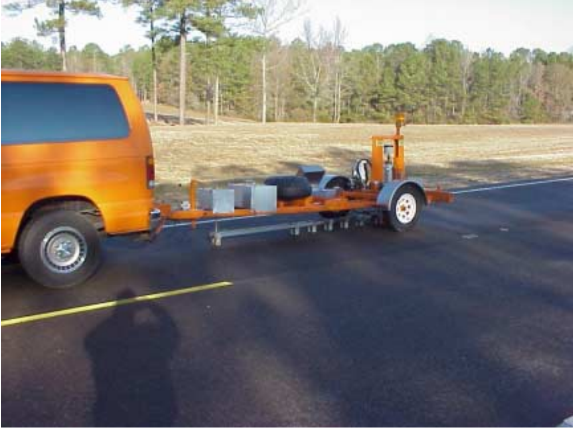
Figure 15. Dynatest 8000 Series Trailer-Mounted FWD Used to Perform FWD Testing
