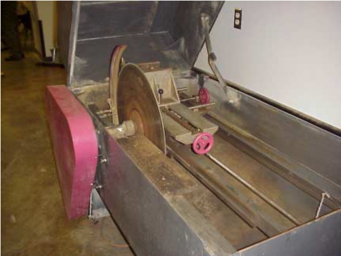
Figure B1. Saw Used to Trim Ends of LFA Cores
