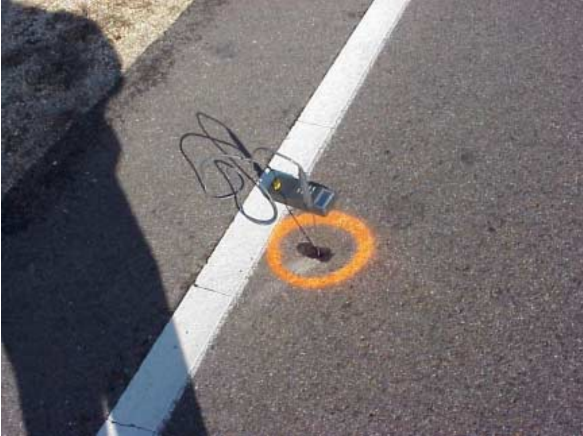
Figure 16. Obtaining Mid-Depth HMA Pavement Layer Temperature
