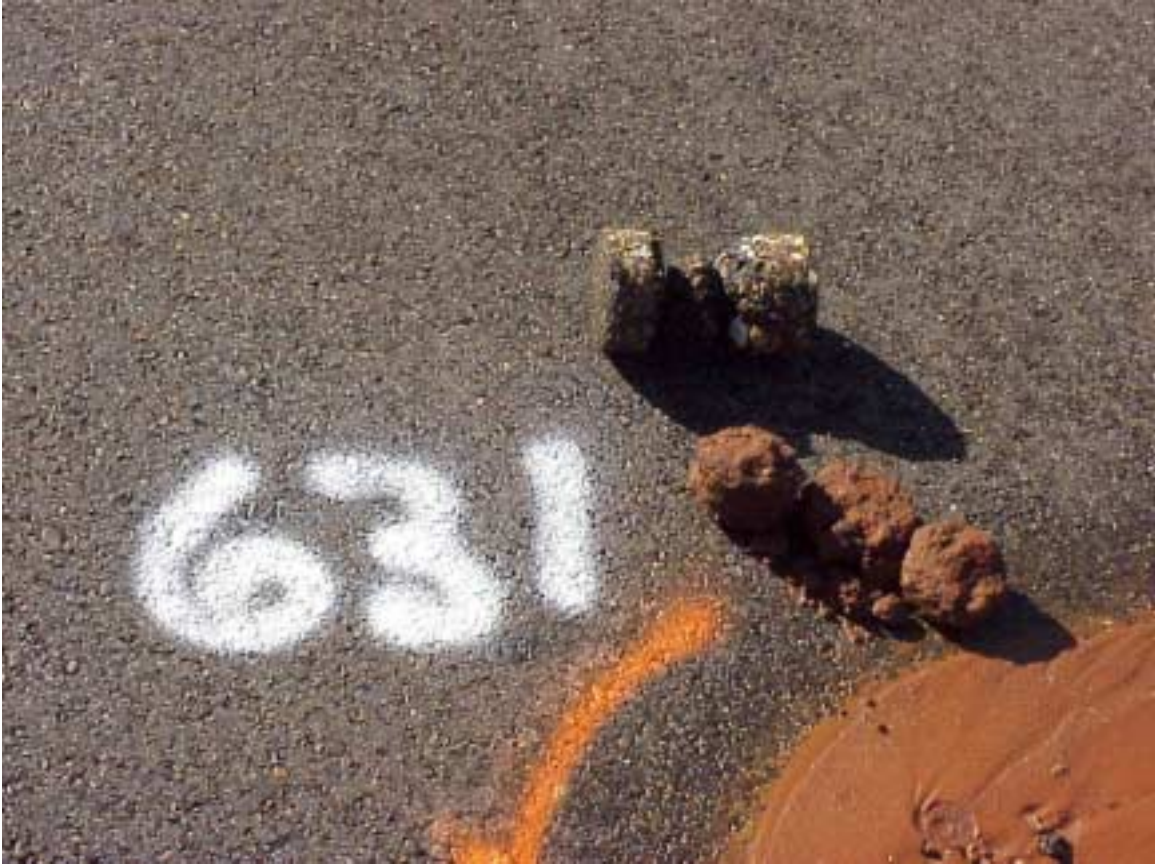
Figure 13. Stripped HMA as Potential Source of Stone for Grooves Cut in LFA Cores
