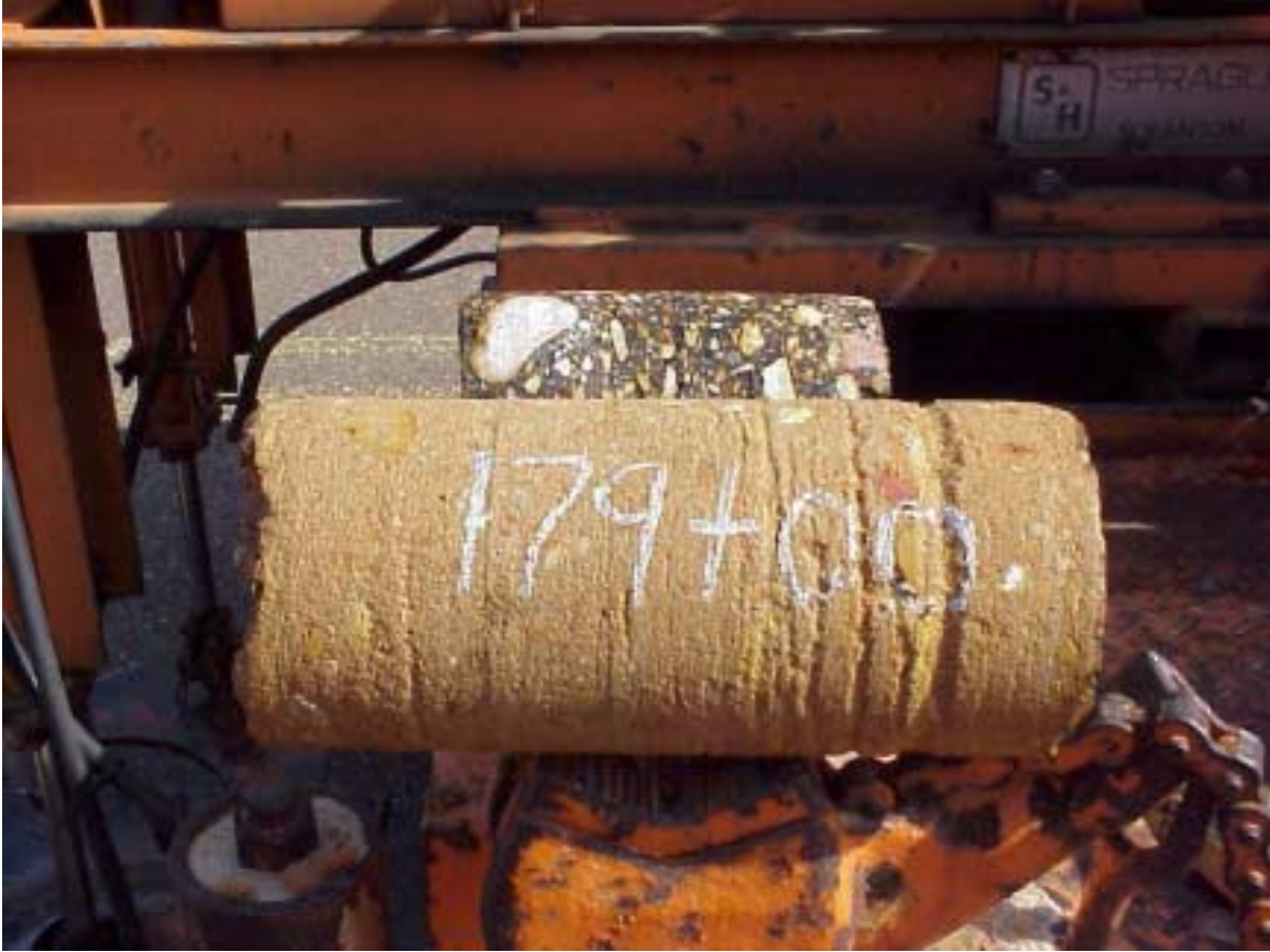
Figure 8. Example of Visual Classification 3—Grooves Cut in Core
