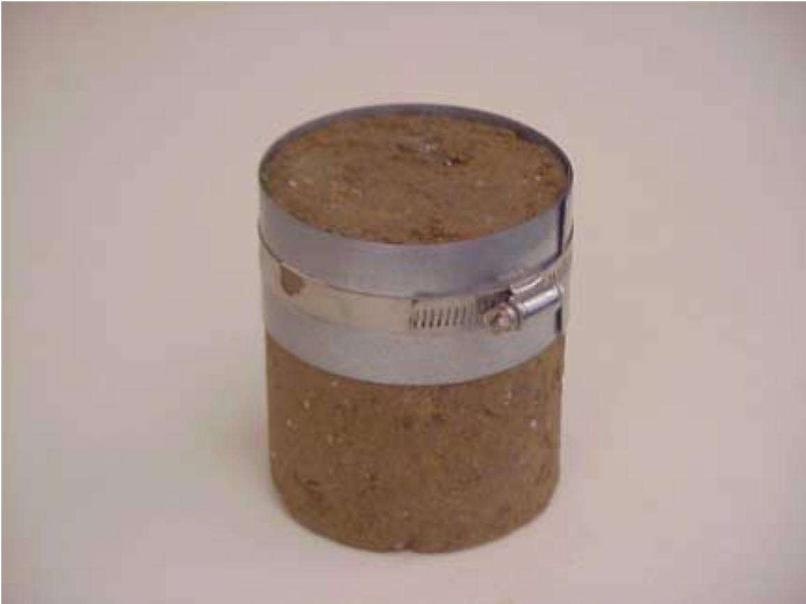
Figure B2. Trimming Ring Used with a Strike-Off Bar to Complete Trimming of LFA Cores
