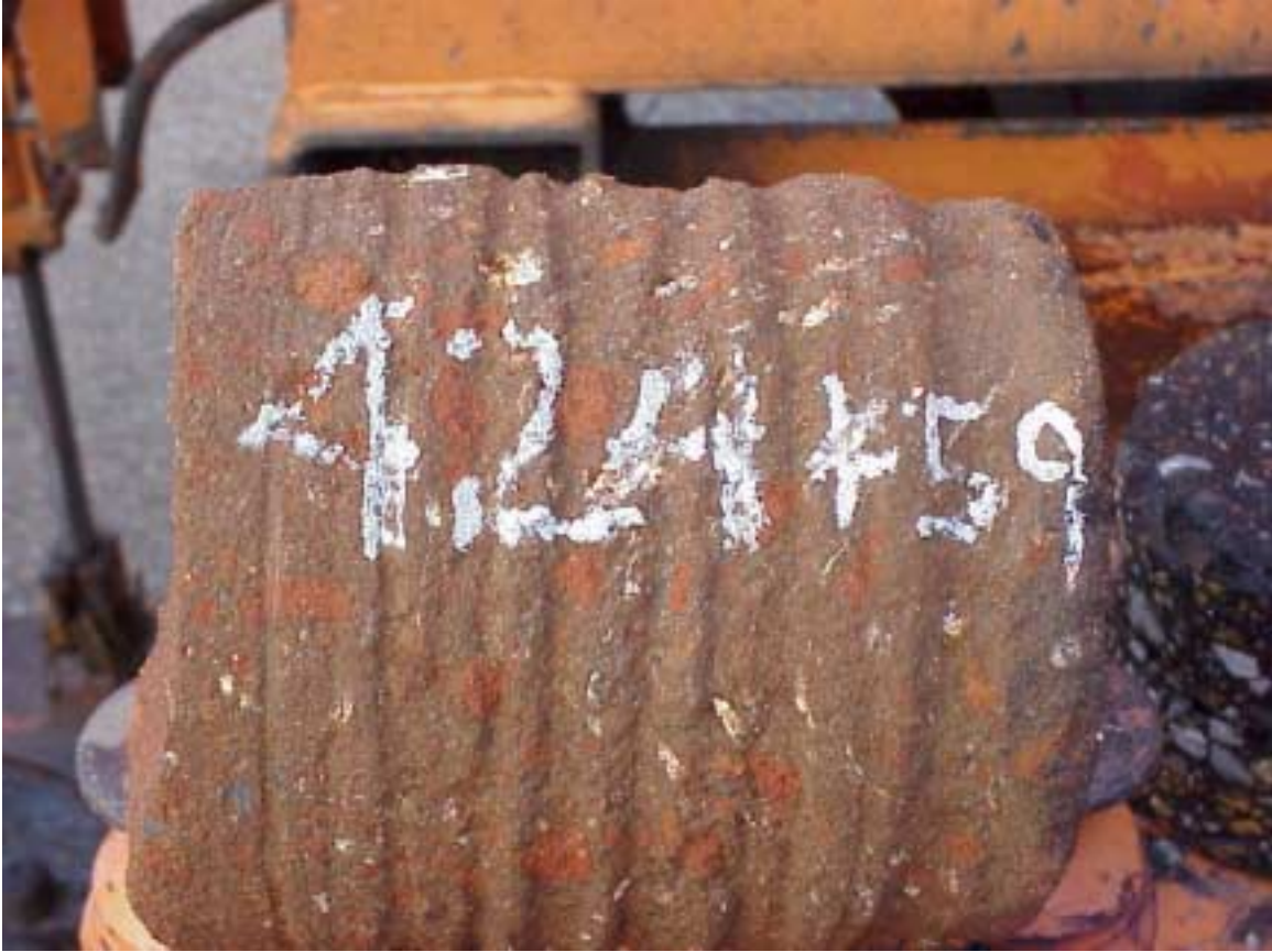
Figure 11. Example of Visual Classification 5—Grooves Cut in Core
