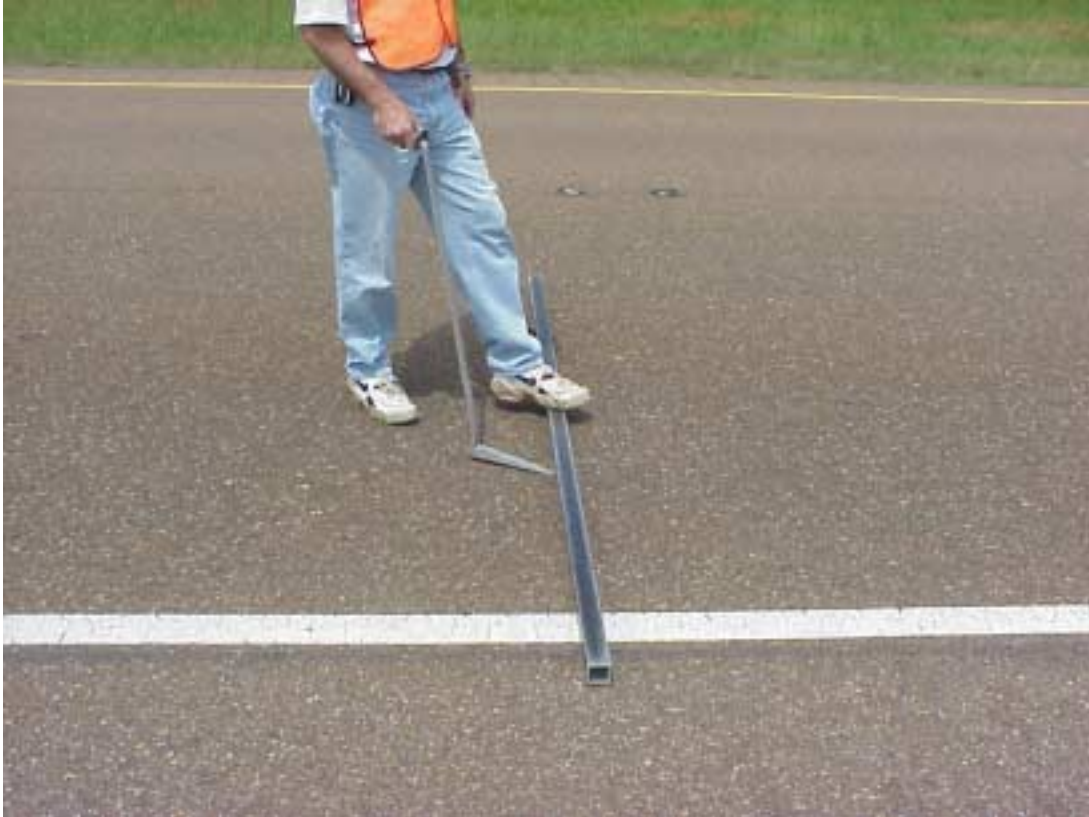
Figure 17 – Manual Rut Measurement
