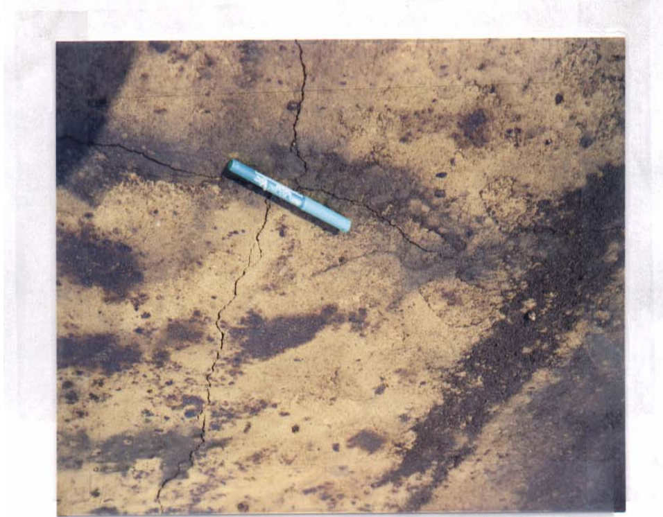
Figure 4.19 Medium severity cracks in section 1A, control cement, fourteenth day.
