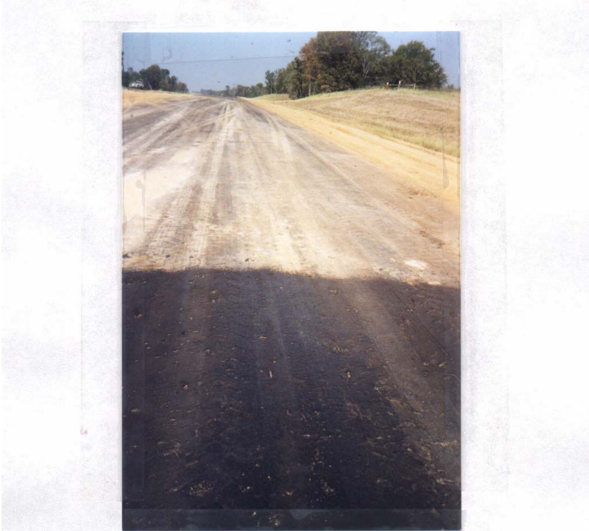
Figure 4.26 Comparison of emulsion retained, section 6 (alternate) in the foreground and section 6 in the background, fourteenth day.
