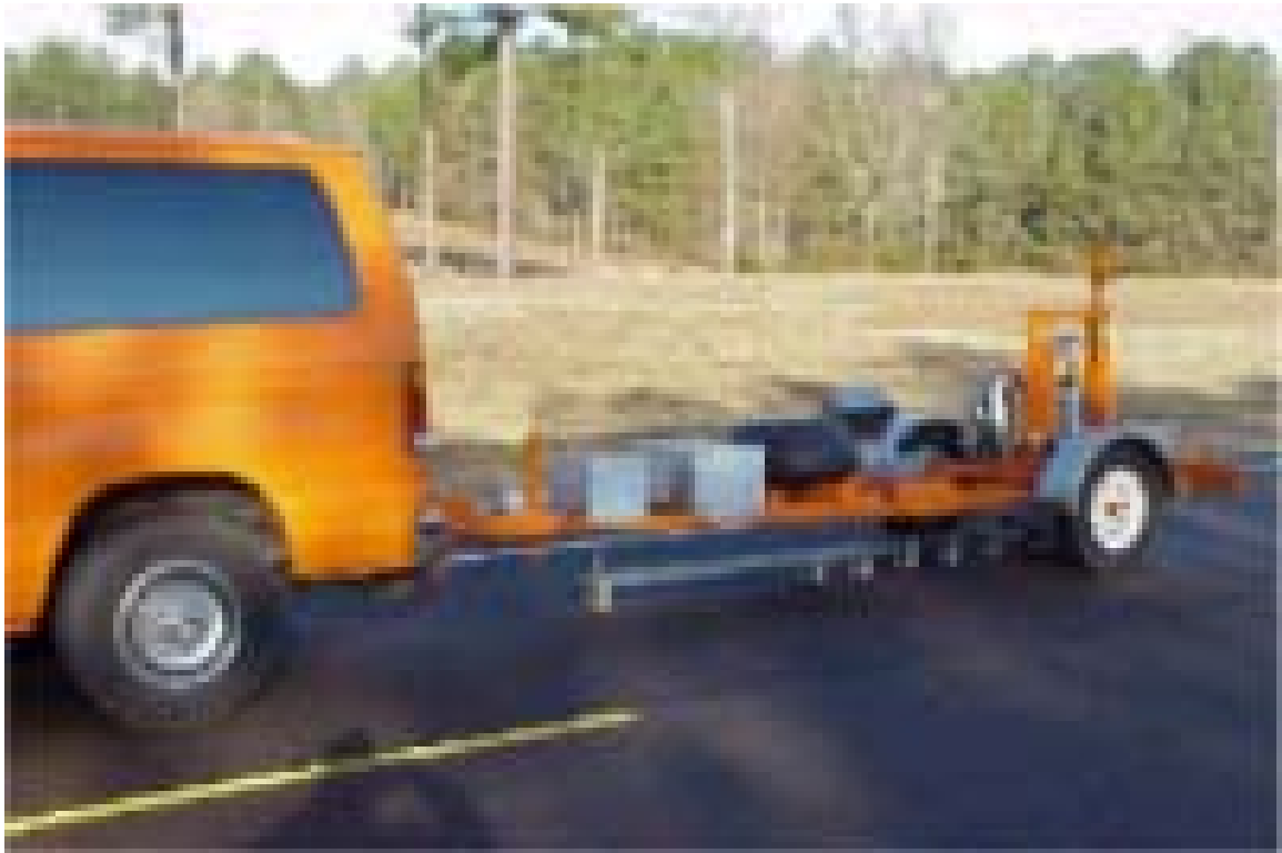
Figure 4.16 Falling Weight Deflectometer in operation.
