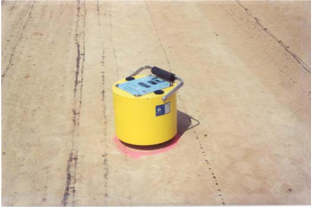
Figure 4.11 Geogauge in operation evaluating modulus of layer in-place.
