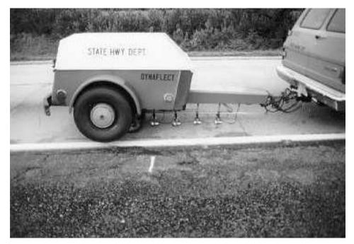
Figure 16. Dynaflect testing.
