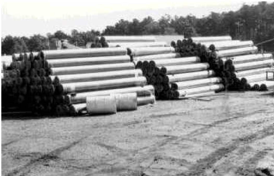
Figure 4. Rolls of moisture barrier fabric.
