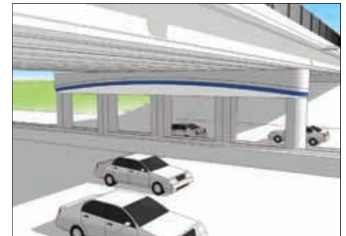
Figure 3.12 – 5 Column Pier without Arched Soffit
