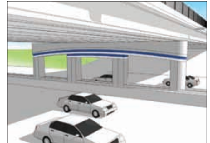
Figure 3.11 – 4 Column Pier with Arched Soffit
