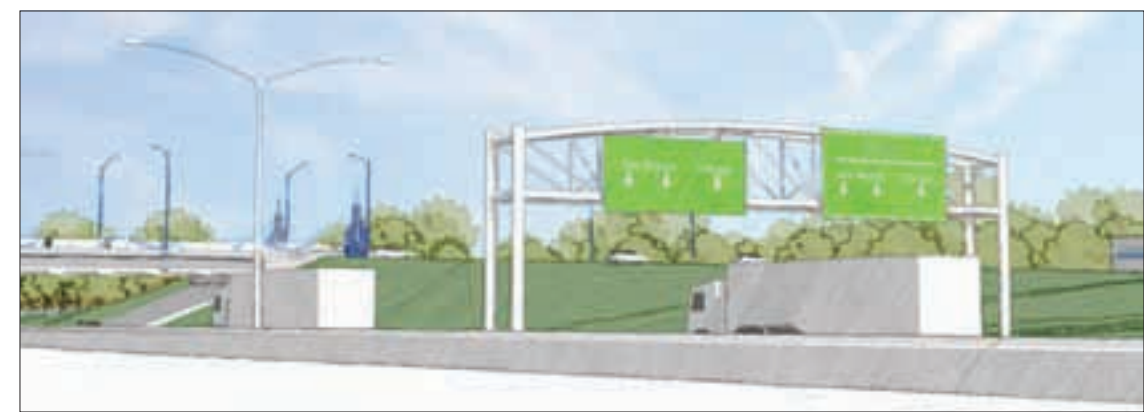
Figure 4.20 – Sign Truss and Lighting Perspective
