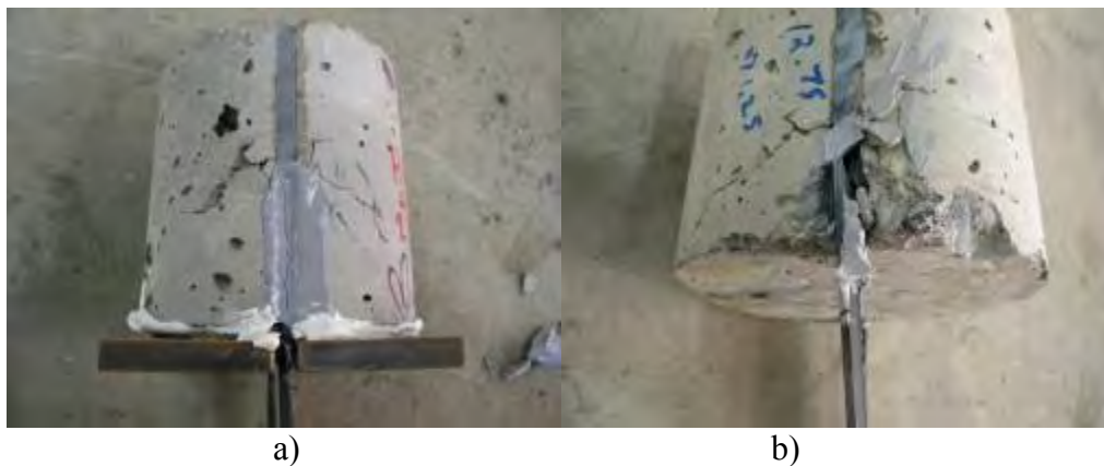
Figure D-9 - Failures of typical C1 specimens
