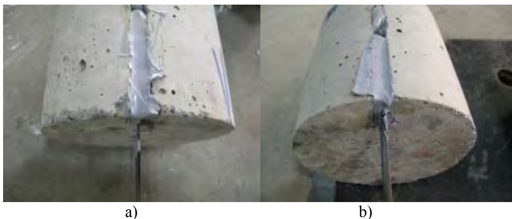
Figure D-10 - Failures of typical C2 and C3 specimens
