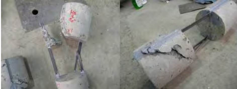
Figure D-2 – Failure of concrete around the NSM repair
