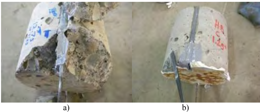
Figure D-12 - Failure of E1.C1.L/4.S specimens
