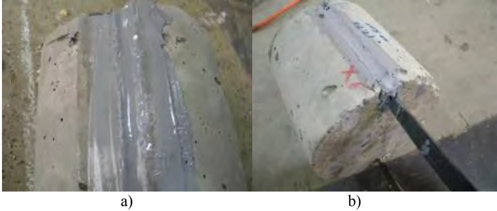
Figure D-11 - Failure of E1.C1.L.S specimens
