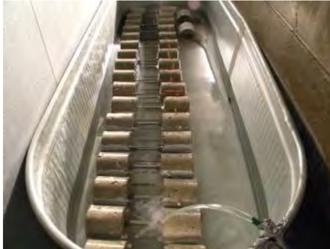
Figure D-4 – Bond specimens subjected to freeze-thaw effects with wet and dry conditions
