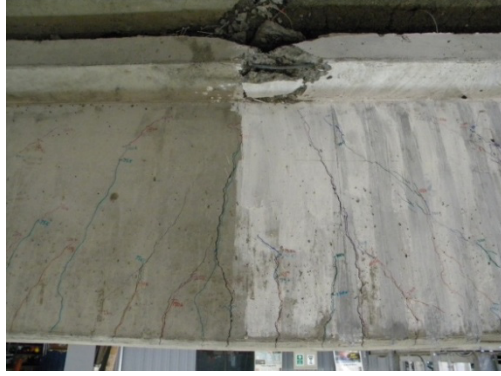
Figure 6.1: Specimen T.6.18.6.S at failure (flexural)
