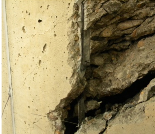
Figure 6.20: Rupture of CFRP strip without slip relative to surrounding epoxy or concrete
