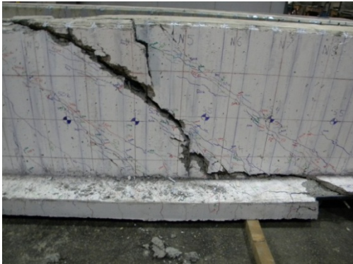
Figure 6.3: Specimen IT.7.18.6.S at failure
