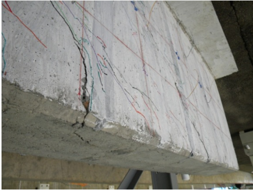
Figure 6.2: Specimen T.6.18.6.S at failure (flexural)
