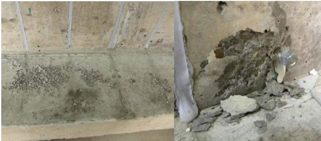
Figure 6.19: Specimen IT.7.22.6.FT effects from freeze-thaw exposure
