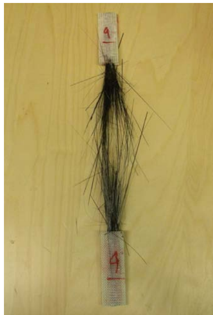
Figure 5.11: Brooming failure of CFRP coupon
