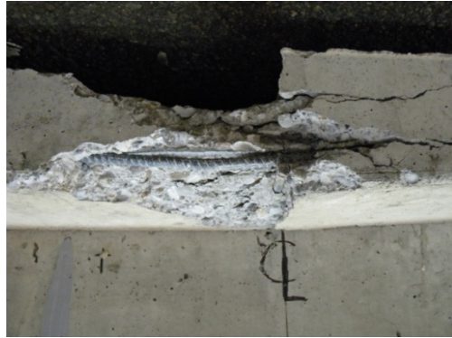
Figure 6.2: Specimen T.6.18.6.S at failure (flexural)
