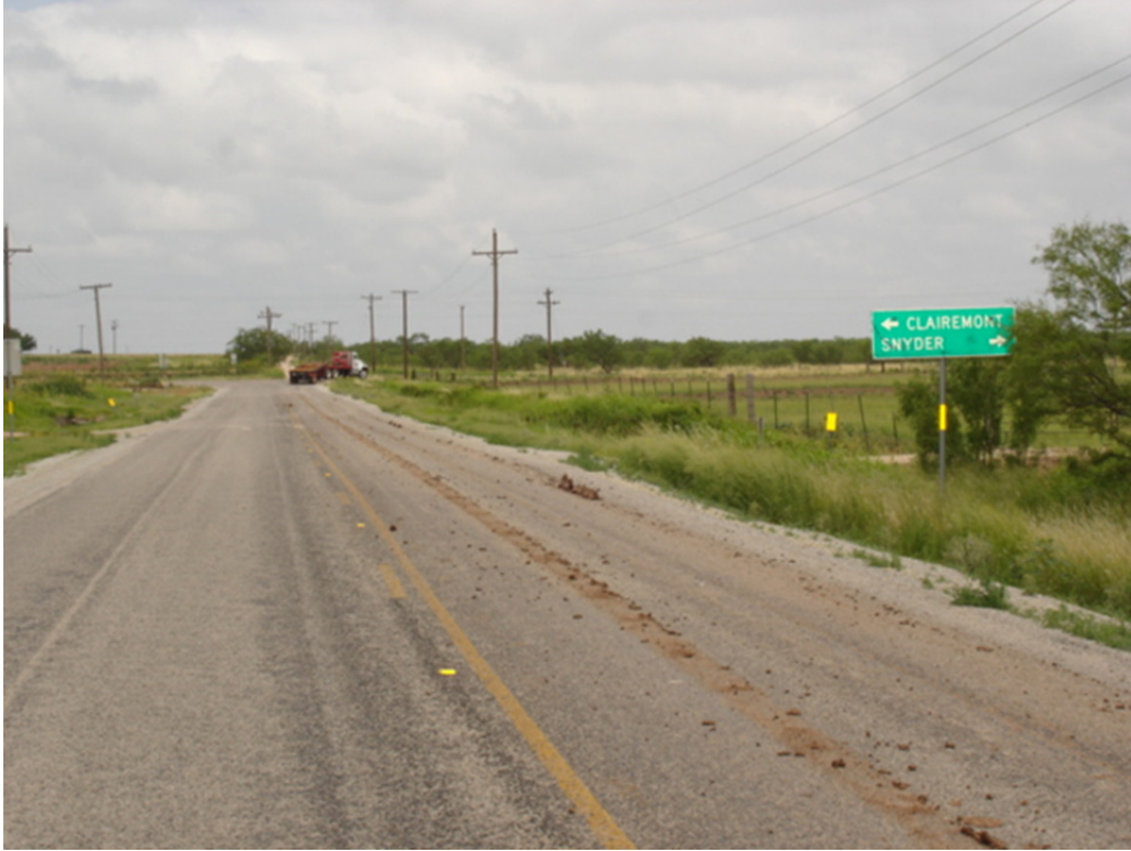
Figure 34. Mud Tracking (FM 1611, Abilene District).
