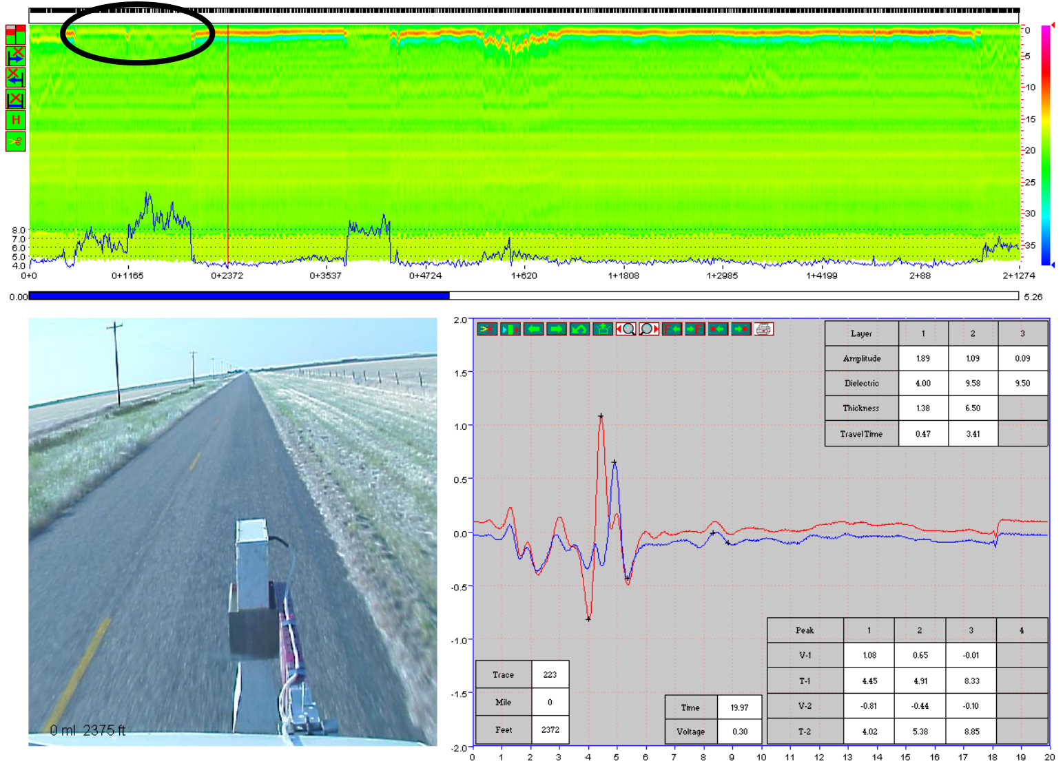
Figure 58. Selection of FWD Test Stations Based on GPR Data Analysis on FM 28.
