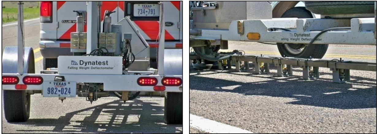
Figure 59. Falling Weight Deflectometer.
