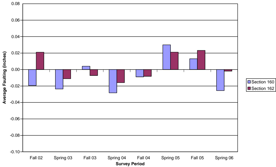
Figure B.3. Faulting, 3.5" depth, patch, no fibers, 4.5' panel
