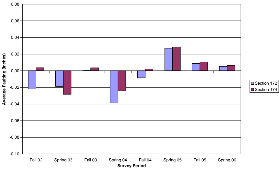
Figure B.35. Faulting, 4.5" depth, patch, fiber A, 6' panel
