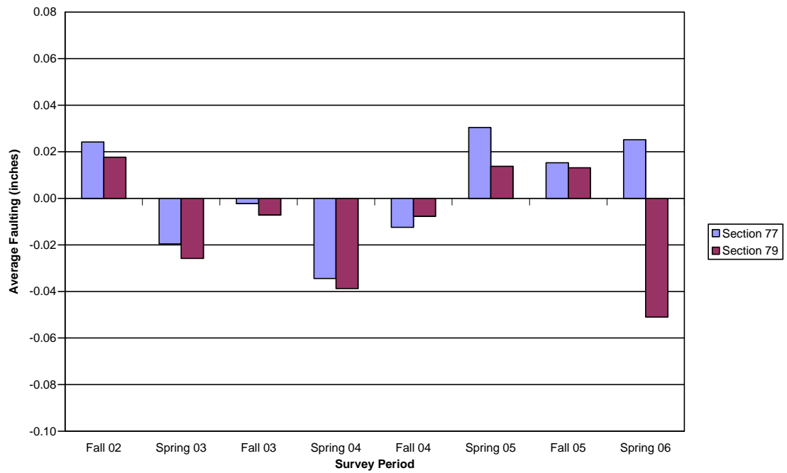
Figure B.15. Faulting, 3.5" depth, HMA S.R., fiber B, 4.5' panel
