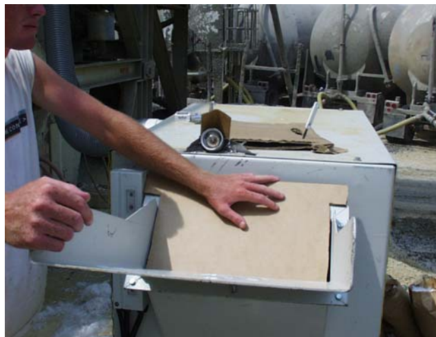
Figure 14. Adjustment to blower for better fiber dispersion
