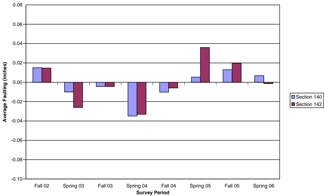
Figure B.13. Faulting, 3.5" depth, patch, fiber A, 6' panel
