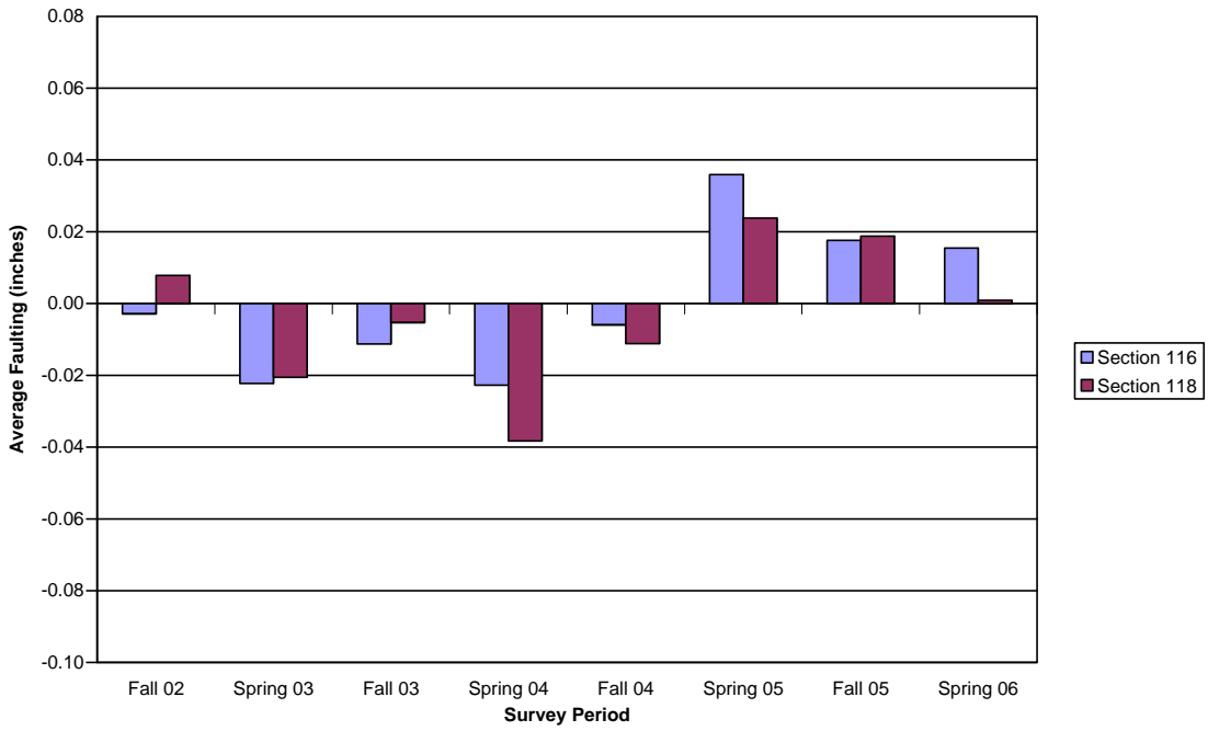
Figure B.40. Faulting, 4.5" depth, HMA S.R., fiber B, 6' panel
