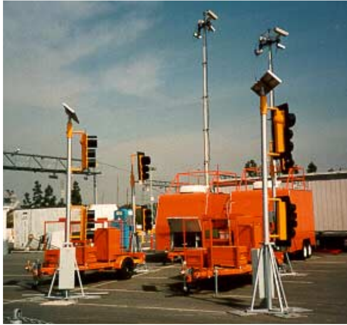
Figure 2-1. Trailer assembly at Hughes in Fullerton, CA showing ramp trailers and signal heads in foreground and surveillance trailers in background
