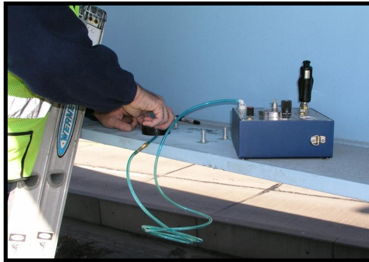
Photo 1, Performing Coating Adhesion Test
