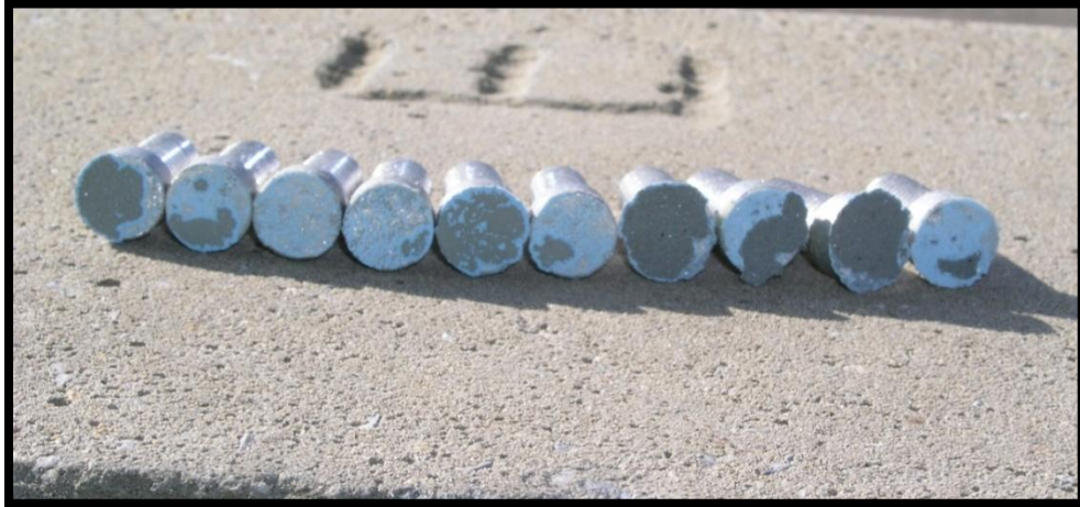
Photo 2, Aluminum test stubs pulled off the coating surface for the Coating Adhesion Test
