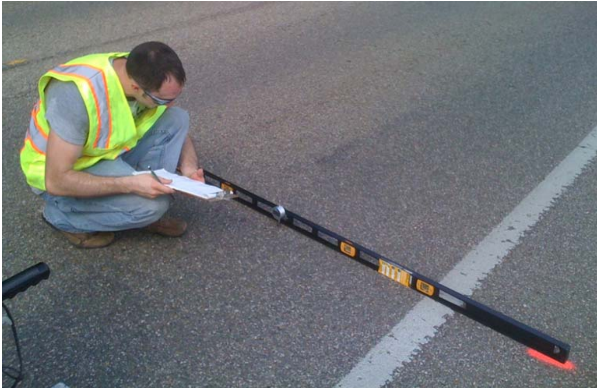
Above: Measuring rut depth with straight edge and dial gauge.
