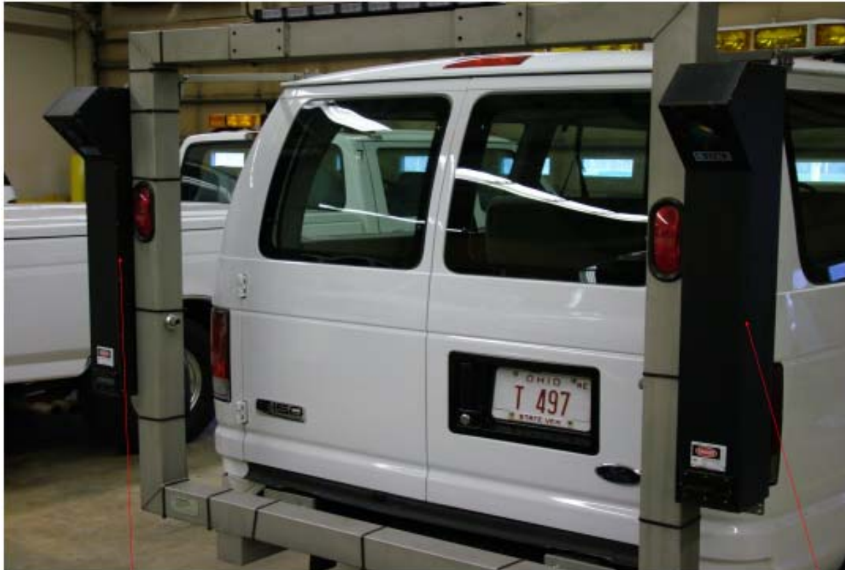
Below: INO Laser Rut Measurement System mounted on Dynatest profiler vehicle.
