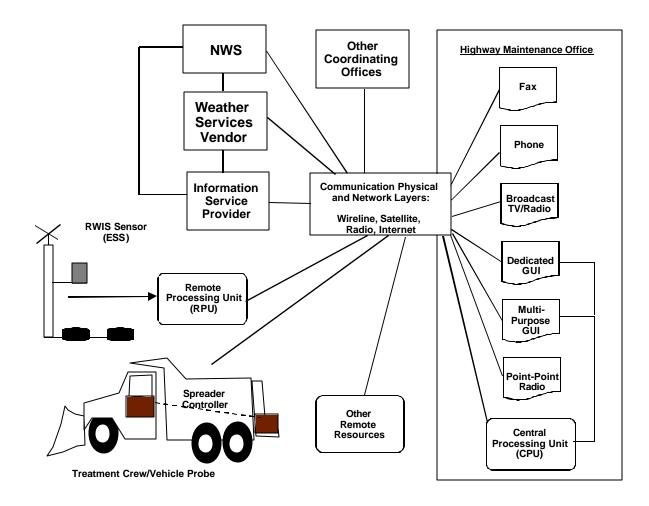
Figure 6.3: RWIS Components and Interconnections
