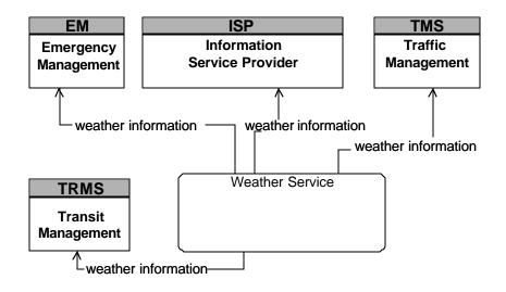
Figure 6.10: Immediate Connectivities to "Weather Service" Subsystem in the National ITS Architecture
