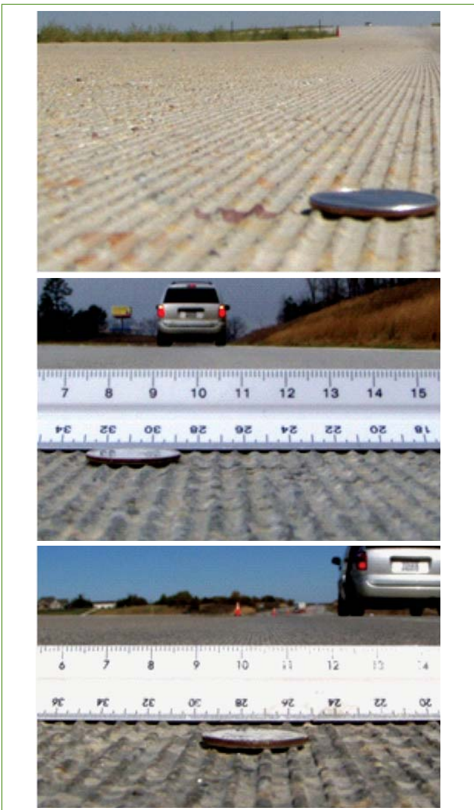
Figure 4. Photographs of quietest diamond ground surfaces – Overall OBSI Level of 97-98 dBA
