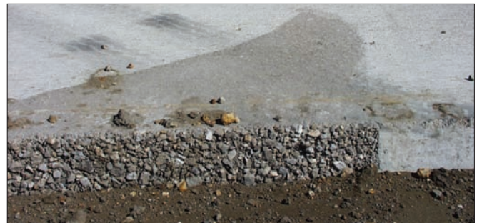
A heavy rain before final set can wash away cement paste and expose course aggregates.
