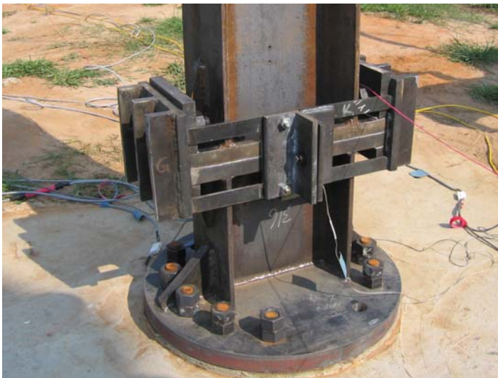
The lower portion of a steel sign post, or stub, extends four inches above the ground. The flange plate at the bottom of the middle post segment rests on the stub flange plate. A multi-part shear-controlled moment collar wraps around and joins the flange plates of the stub and middle post.
