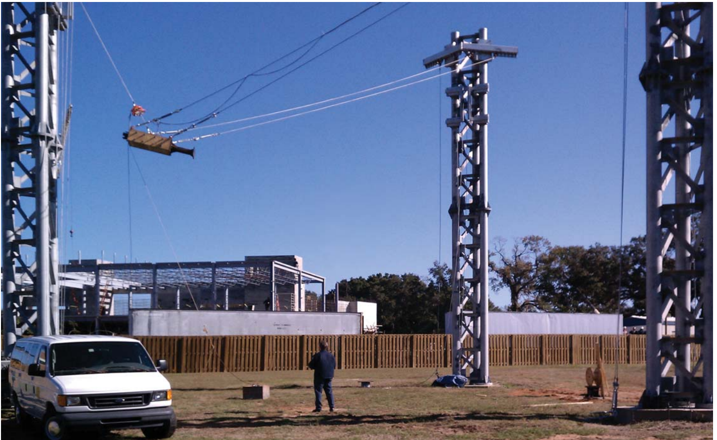
The pendulum impact apparatus located at FDOT's Marcus H. Ansley Structures Research Center in Tallahassee, Florida, consists of three 50-foot towers arranged in a triangular configuration and an impact block. An electric winch hoists the impact block to the desired height. The pendulum is capable of swinging a block weighing up to 9,000 pounds (the weight of two full-size pickup trucks). Upon release, the block can drop through a maximum height of 35 feet and accelerate to a maximum speed of 32 mph at the bottom of the swing.
