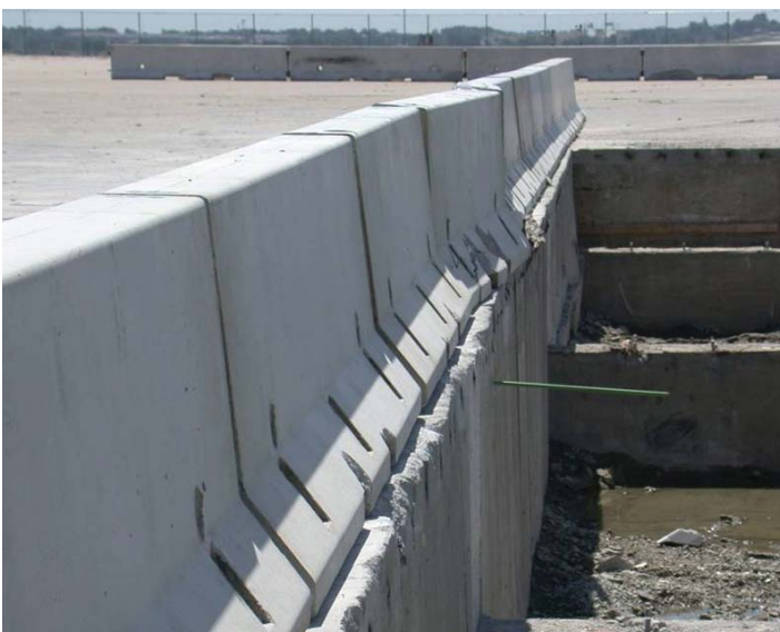
Above: Close-up view of K-barrier damaged in the MwRSF crash test.
