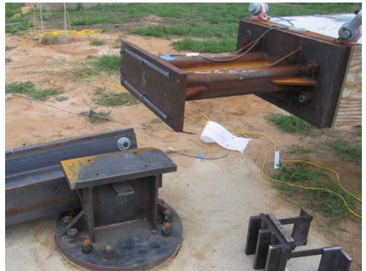
After the impact test, the front half of the moment collar lies on the ground, bottom right; the back half of the collar traveled several feet in the direction of impact as anticipated.
