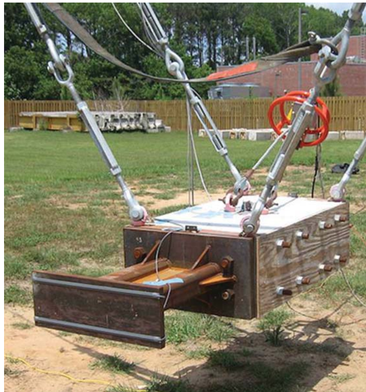
The pendulum impact block fitted with a rigid nose and equipped with tape switches to record the instant of impact. The pendulum supports impact blocks of varying weights, which can be fitted with either rigid or crushable impact noses, depending on the nature of the test.
