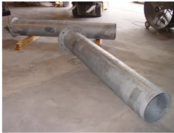
Figure 3-10. Tapered steel poles manufactured by Valmont Structures. Photo courtesy of FDOT.
