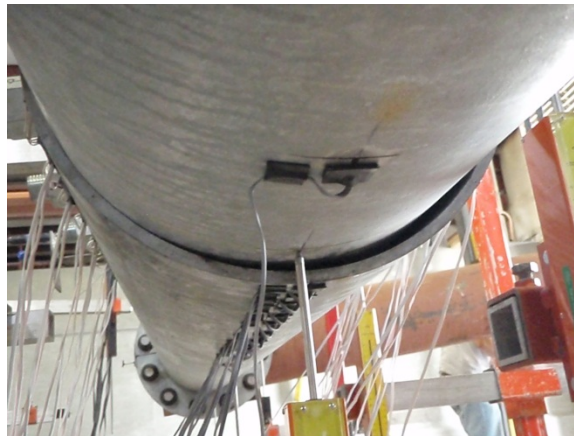
Figure 5-11. Oblong deformation at the base of the outer pole during loading. Photo courtesy of S. Dalton.
