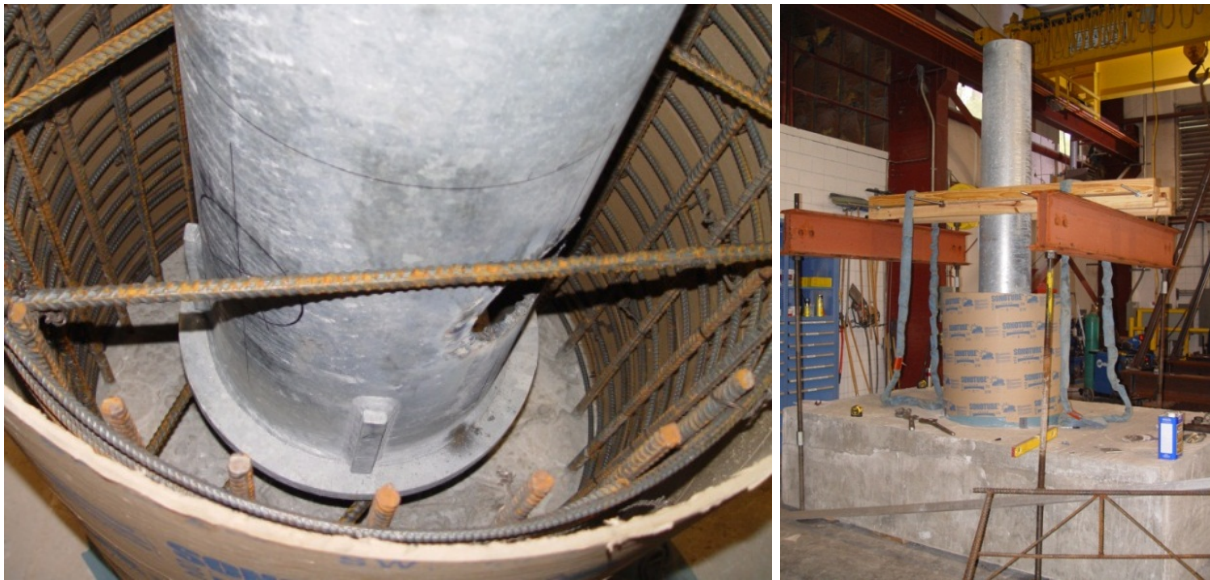
Figure 6-1. Alignment rebar within pedestal and external bracing of embedded pole. Photos courtesy of FDOT.
