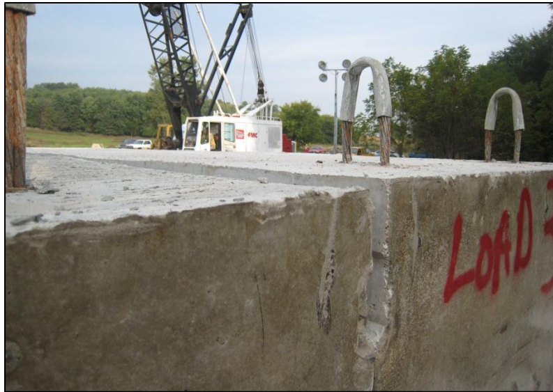
e. Difference in beam thickness
