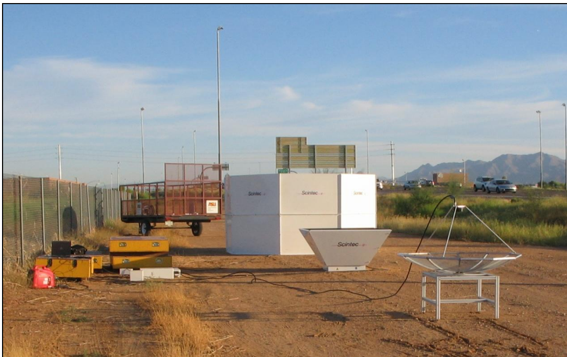
Figure 5. Photographs of instruments deployed in the experiment. Two sonic anemometers on a short tripod on right side, and two microphones on the tripod in the left side of the picture, at Loop 202 in November 2006 (top); and the SODAR-RASS system at Loop 101 in October (bottom).
