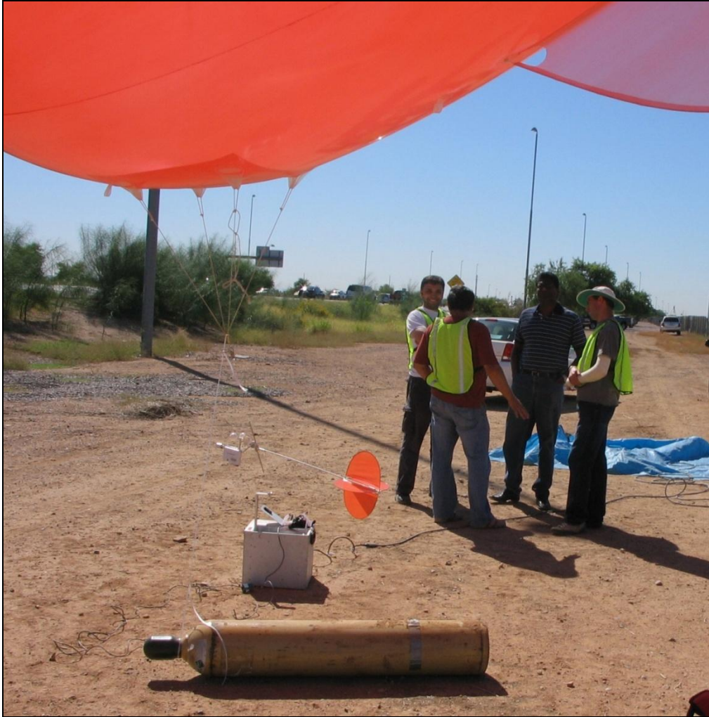
Figure 6. Photograph of the balloon-tethersonde system used at the Loop 101 site in October 2006.
