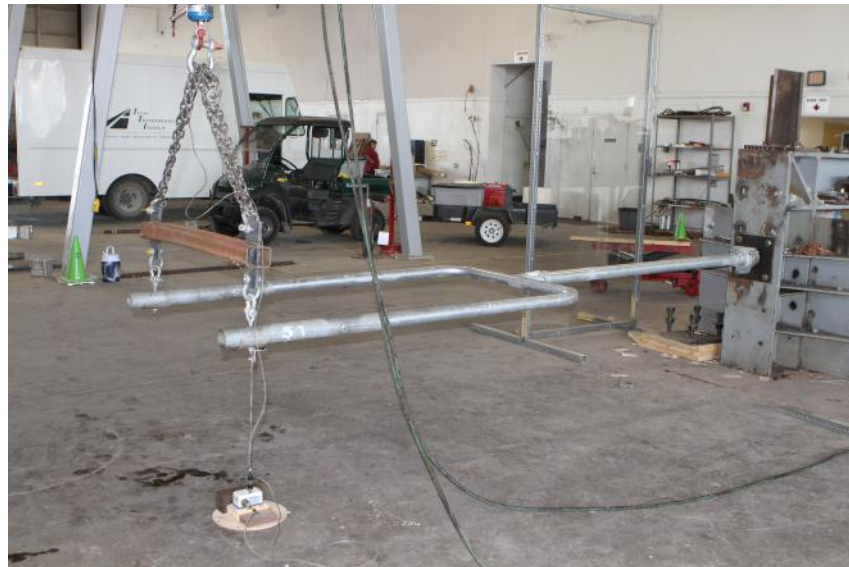
Figure 11.10. Image of U-Bracket Installation Static Test Setup prior to Loading.
