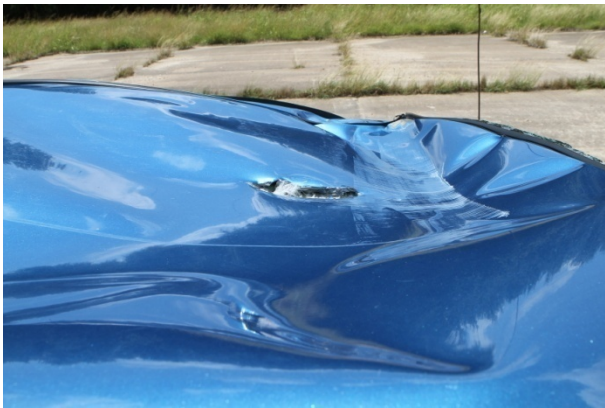
Figure 9.42. Vehicle Roof Deformation after Test No. 463631-2.
