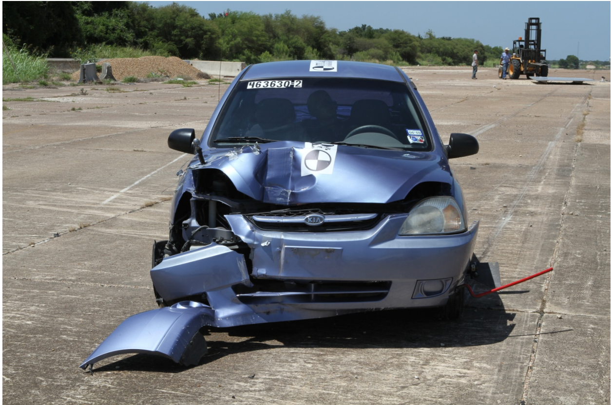
Figure 7.30. Vehicle after Test No. 463630-2.
