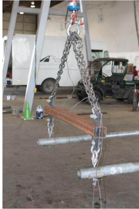
Figure 11.11. Image of U-Bracket Load Application.
