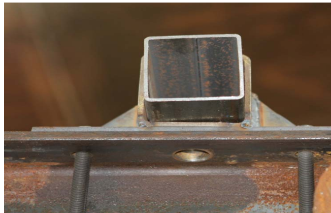
Figure 7.9. Static Test of HSS3×3×1/8 with Bracket Connection.
