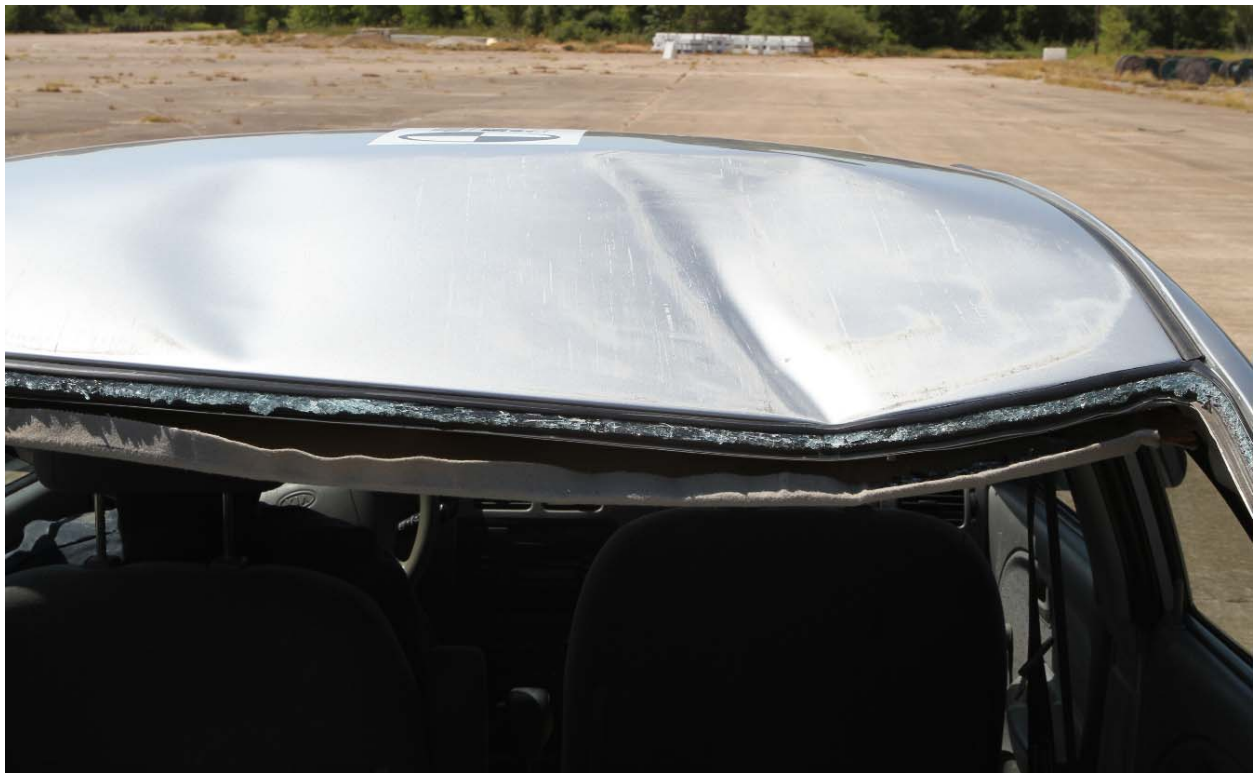
Figure 9.58. Vehicle Roof Deformation after Test No. 463631-3.
