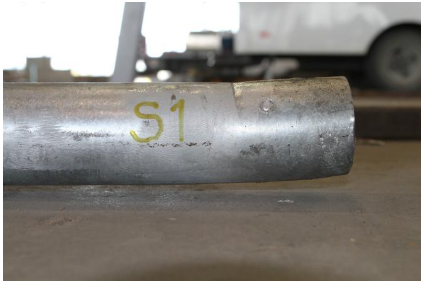
Figure 11.12(b). Image of Deformation to Schedule 80 Pipe Support.
