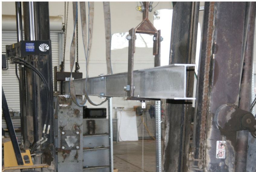
Figure 5.12. W8×18 Support Ready for Load Application (S3).
