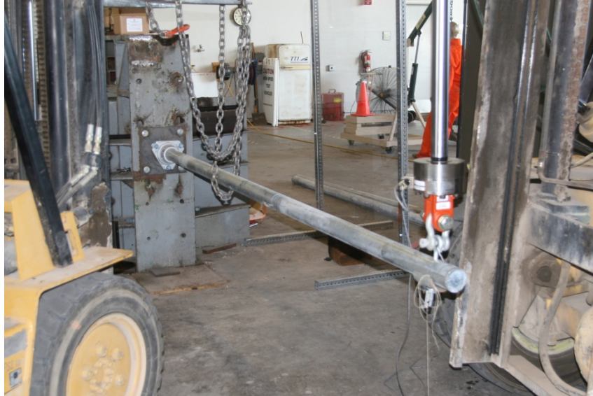
Figure 3.2. Schedule 80 Support Static Testing Setup before Load Application.
