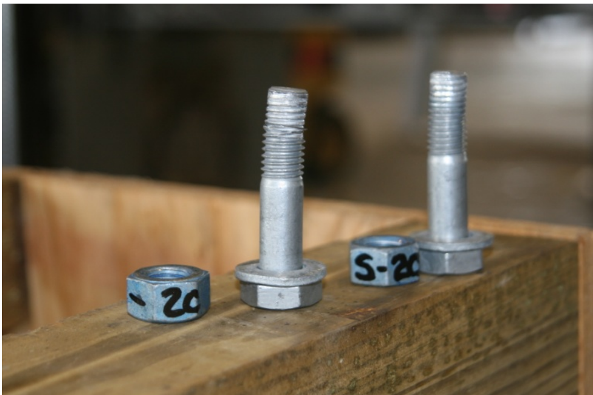
Figure C8. Slip Bolts after Test S20.
