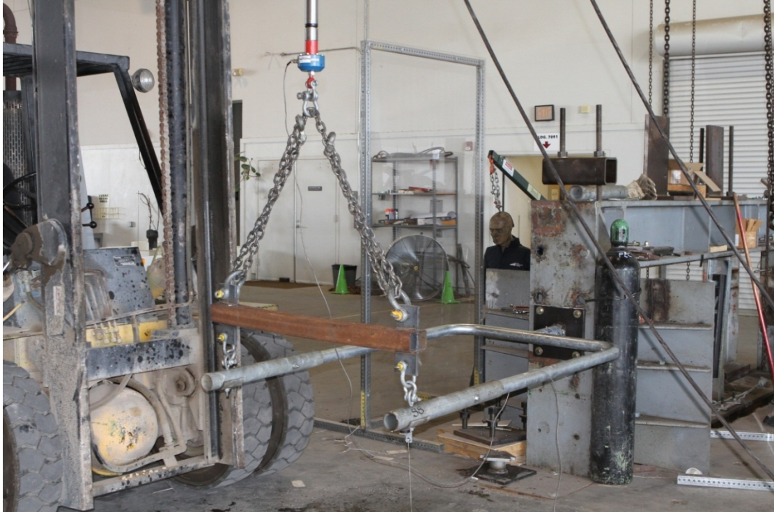
Figure 11.19. U-Bracket Static Test Setup prior to Loading.
