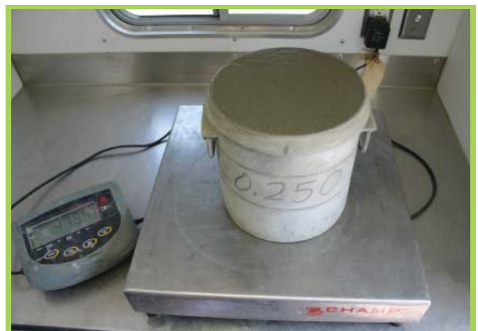
Figure 7.23 Unit weight test equipment
