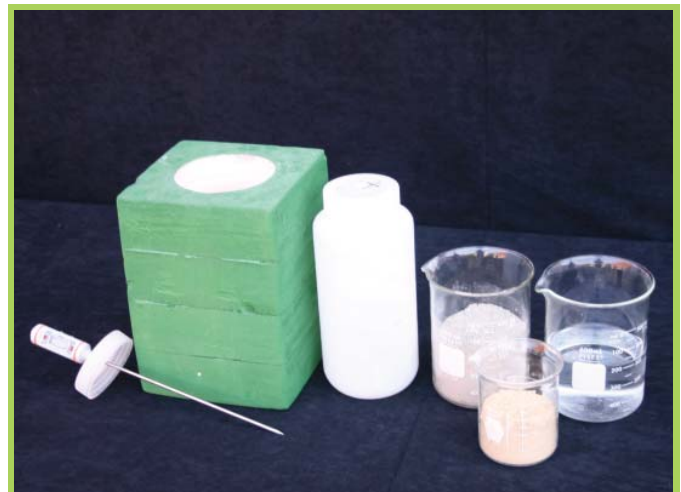
Figure 7.12 Cementitious heat generation test equipment and materials
