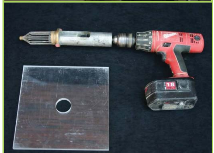
Figure 7.26 AVA setup in a portable lab and AVA sampling equipment
