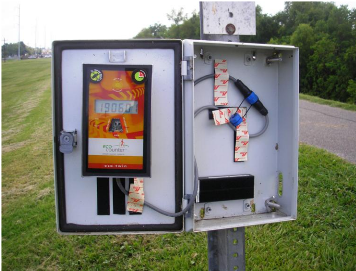
Figure 3.2.1 Eco-Counter box at Mississippi River Trail
