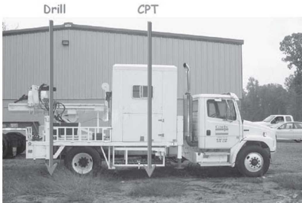
Figure 7.5. CPT rig with drilling capabilities (Mayne 2007)
