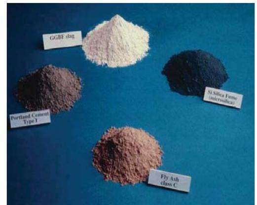
Another benefit of replacing Portland cement with fly ash and slag is a reduced carbon footprint during production of the cementitious material. Production for each ton of Portland cement for concrete pavement emits 0.92 tons of carbon dioxide. As byproducts of other industries, emissions due to production of fly ash and slag are negligible from the viewpoint of concrete pavement construction.
