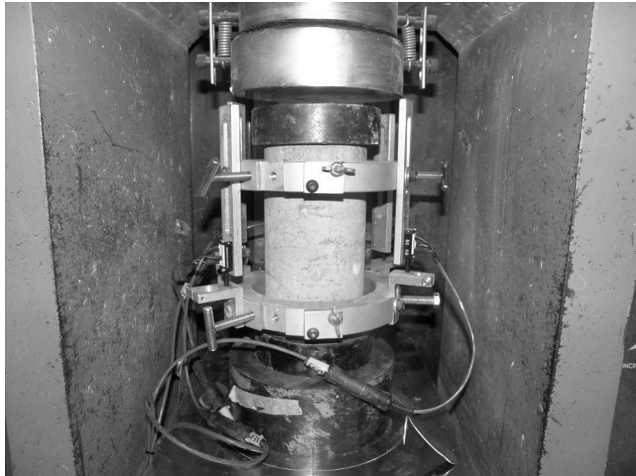
Figure E-1 Test setup for elastic modulus testing of concrete cylinders.
