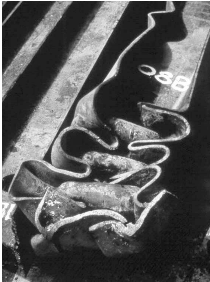
Figure 1.7. Damage to steel piles due to excessive driving hammer size (Salgado 2006)
