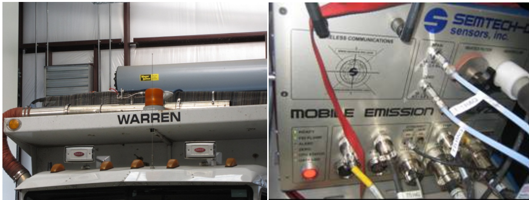
Figure 8. SEMTECH EFM Installed on Test Vehicle (Left) and SEMTECH-DS (Right).
