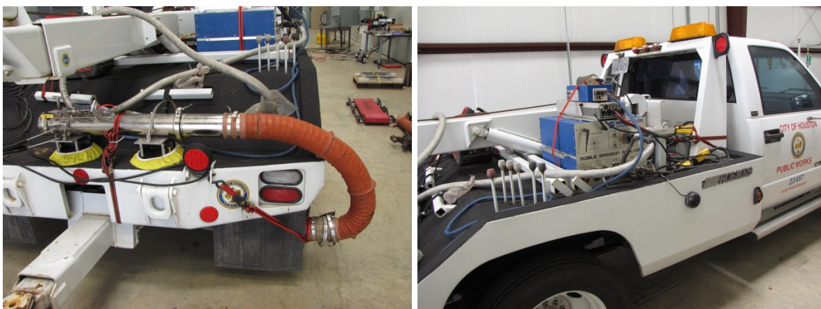
Figure 4. Class 4 Vehicle Instrumented for Testing.
