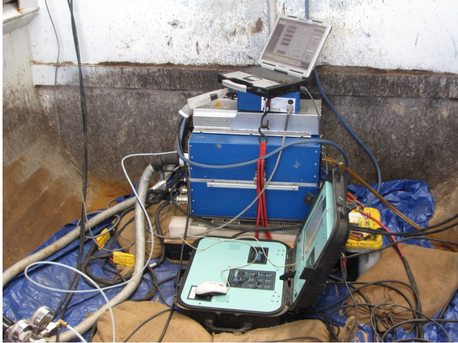
Figure 9. CATI Axion System along with the SEMTECH-DS Installed on Test Vehicle prior to Testing.
