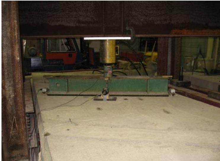
a) Laboratory setup for line load ultimate load test
