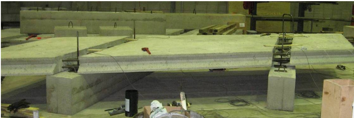
Figure 2.14. Deck panel setup for leveling test
