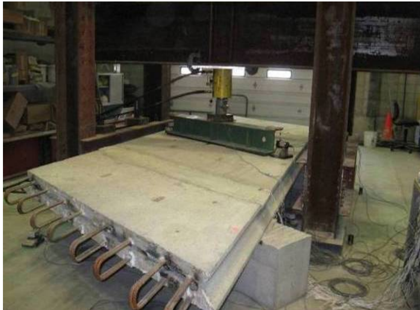
b) Panel 3 setup prior to testing
