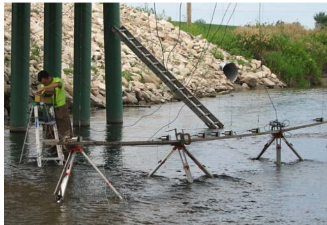
Figure 2.3 Tripod system used to support displacement transducers
