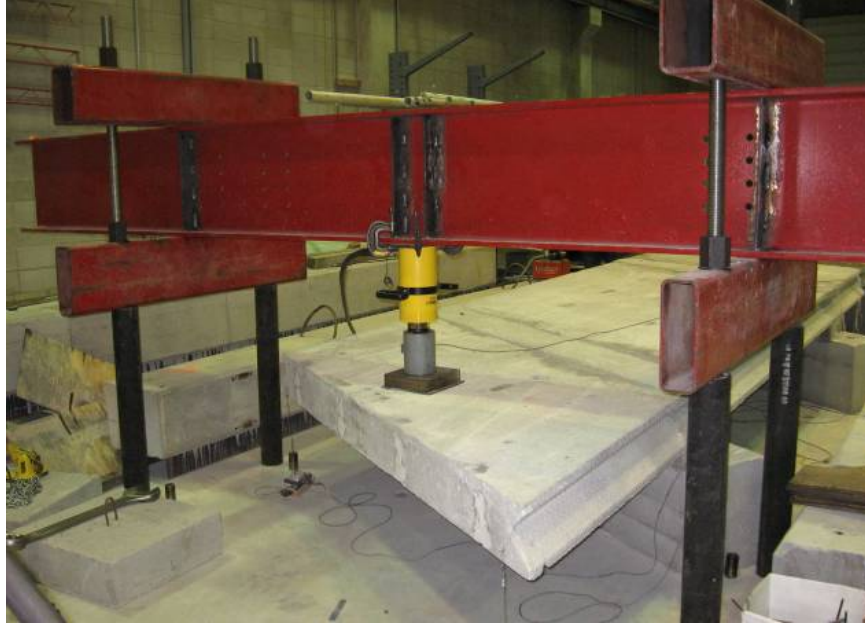
a) Service load at Position B2
