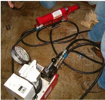
a) Mono-strand jack and hydraulic pump
