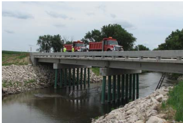
Figure 2.11 Static test (Load Case 1)
