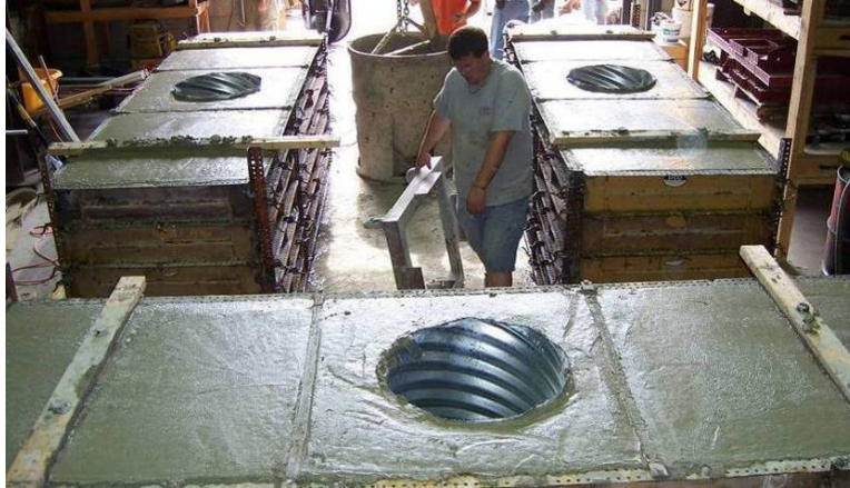
Figure 20. Hand-finished specimen before initial set
