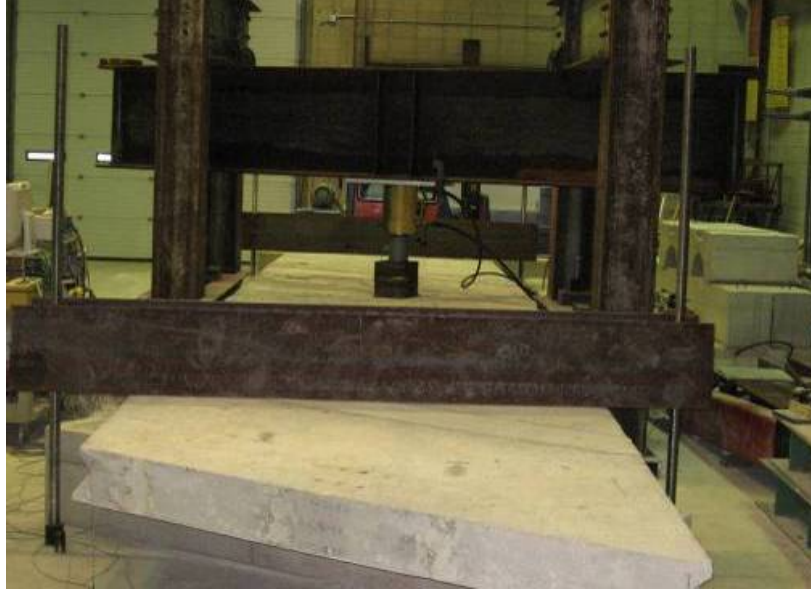
c) Restraining beams positioned for ultimate load test
