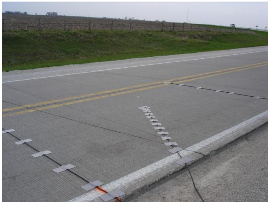
Figure 3.6. Road tube layout to measure lateral displacement in the field
