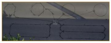
Loop detector test bed.
