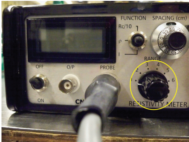
Fig. 1 The resolution switch (noted in yellow) can be moved to increase/decrease the resolution of the display
