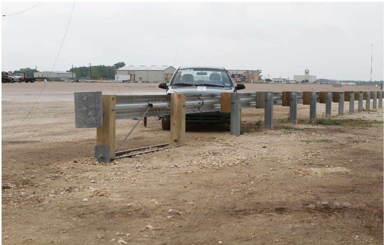
Figure 5.1. Vehicle/Installation Geometrics for Test No. 420021-1.
