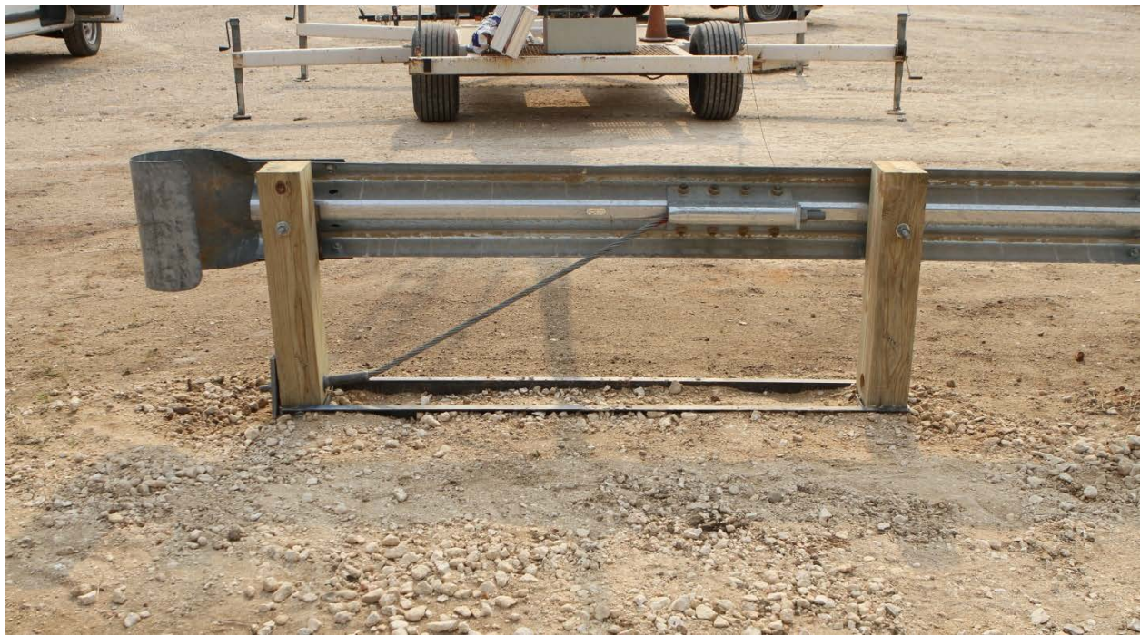
Figure 2.2. TxDOT 31-inch W-Beam Downstream Anchor Terminal before Test No. 420021-1.
