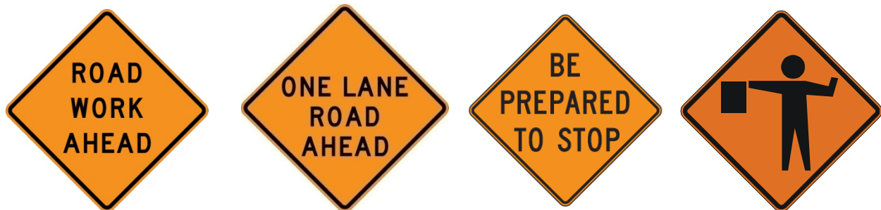
Figure 10. Phase 1 Advance Warning Signs.
