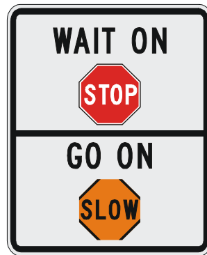
Figure 14. Alternative Supplemental Sign for Stop/Slow AFADs.
