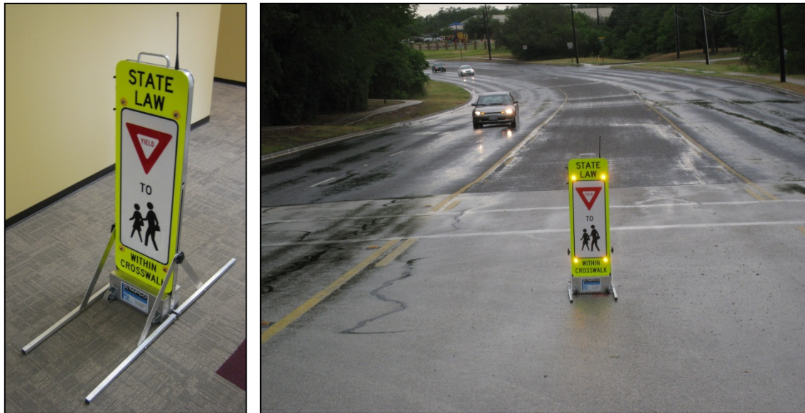
Figure 26. Prototype LED Enhanced In-Street School Crossing Sign.
