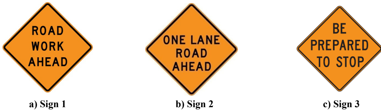
Figure 13. MUTCD Recommended Advance Warning Sign Sequence.
