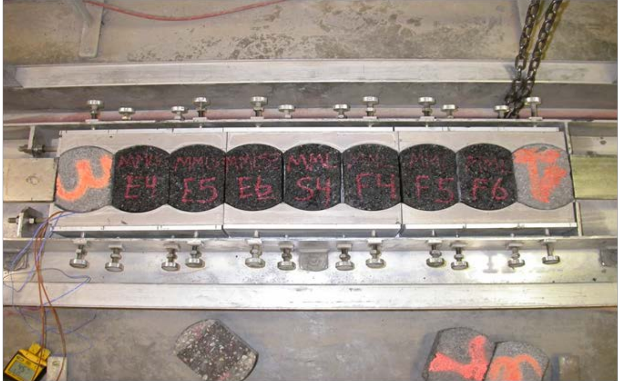
Figure 11. Trimmed SGC Specimens Arranged for MMLS3 Tracking
