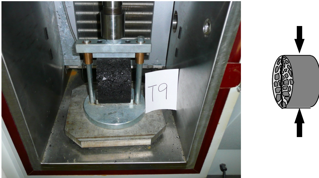
Figure 10. SGC Specimen Set in the Loading Frame for Indirect Tensile Testing and Corresponding Loading in Diametral Direction
