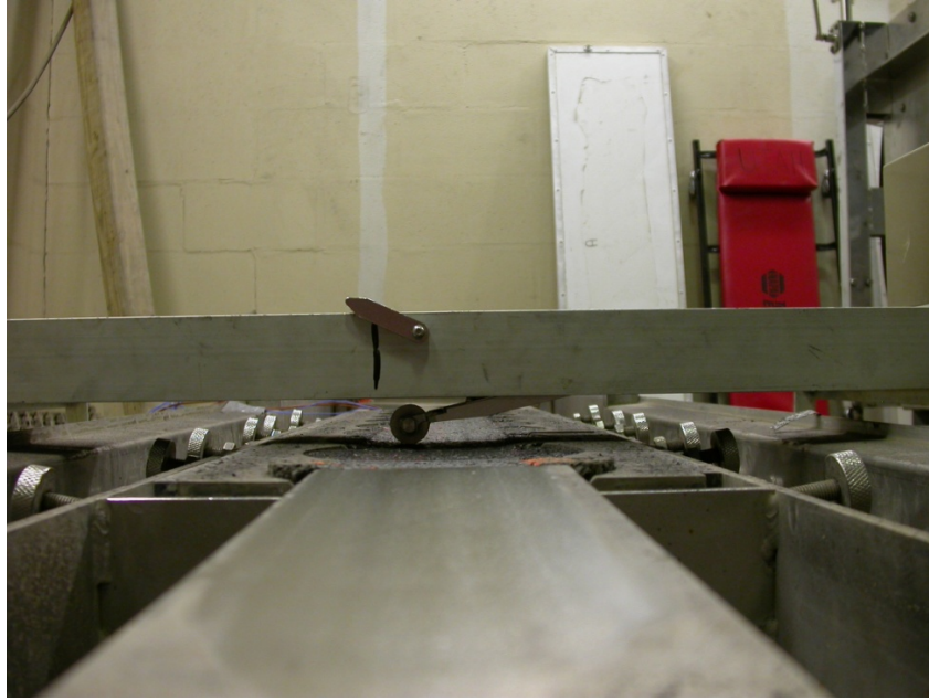
Figure 14. Profilometer Used to Measure Rut Profiles
