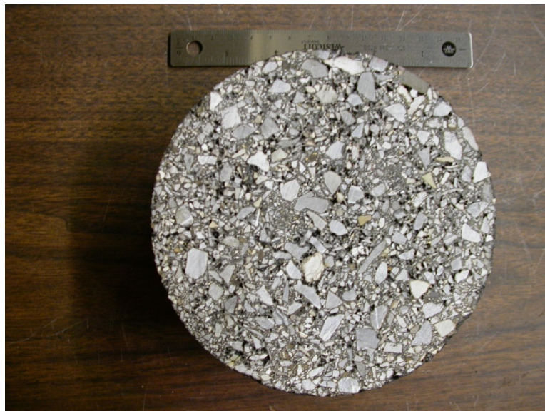
Figure 16. Sawed Face of 6-inch SGC Specimen for SST
