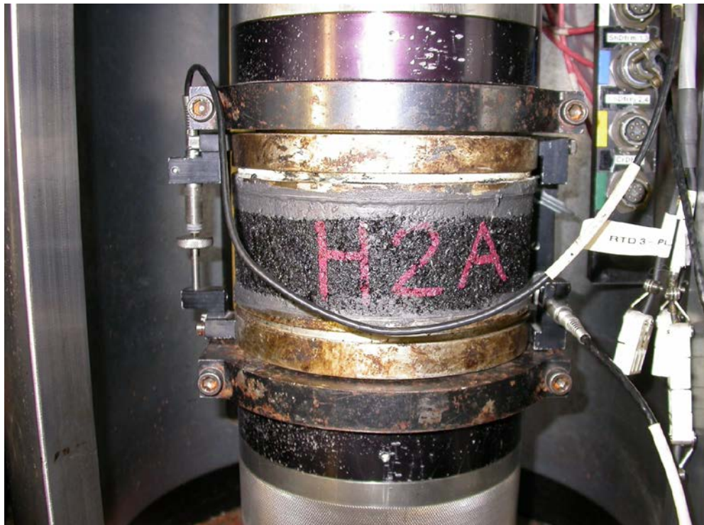
Figure 18. Assembly of Specimen and LVDTs for Deformation Measurement
