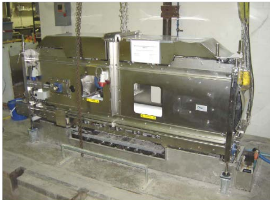
Figure 12. MMLS3 Loading System Assembled and Ready to Load Specimens
