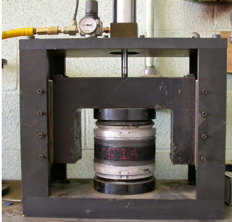
Figure 17. Gluing Jig for Fixing Platens to the Shear Test Specimen
