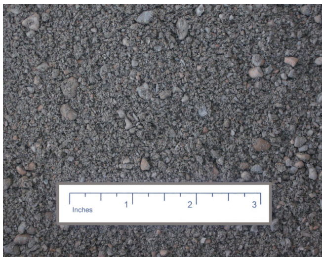
Figure 4.8 Light-weight fine aggregate (image courtesy of Buildex)
