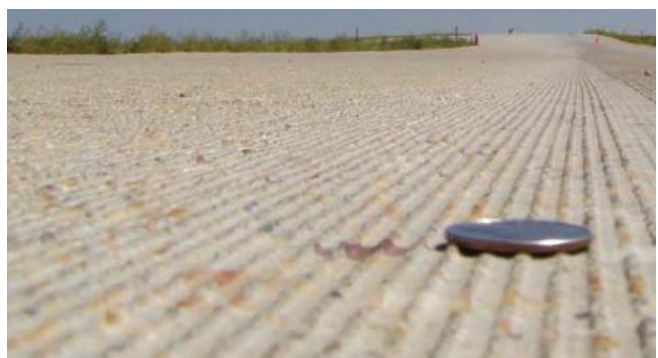
Figure 5.11 Diamond-ground texture (Rasmussen et al. 2008)
