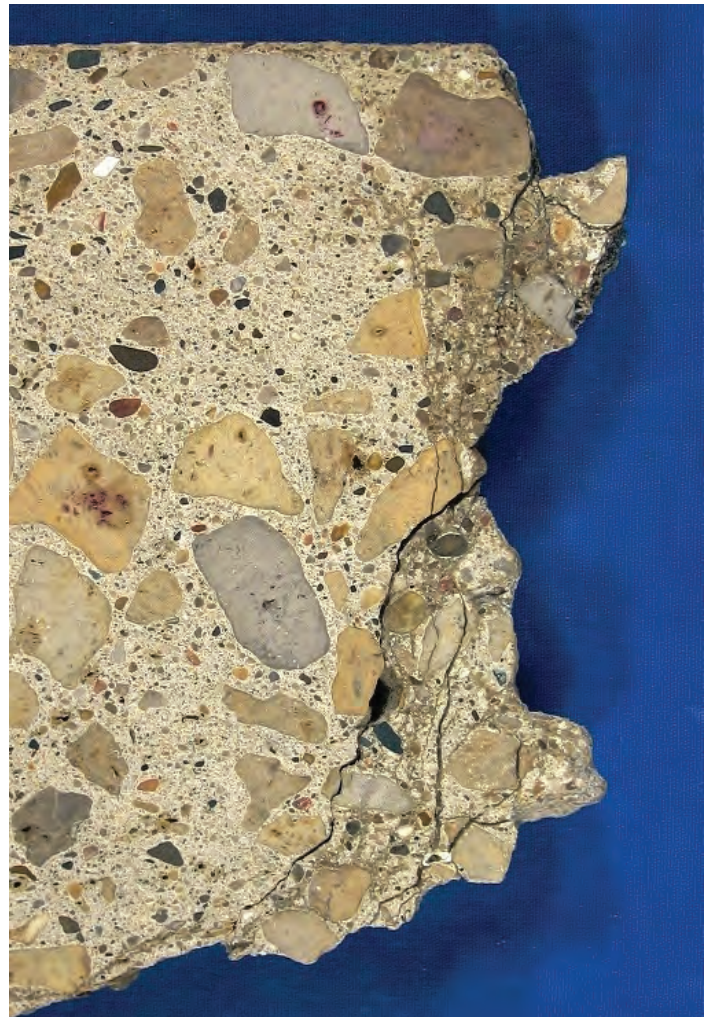
Figure 21. Deterioration due to bottom-up moisture
