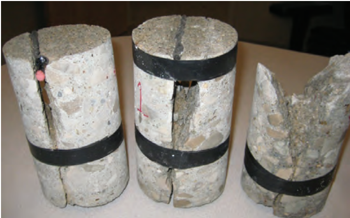
Figure 12. Three cores illustrating progression of distress from bottom-up moisture
