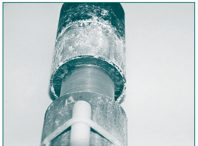
Figure 14. Zinc alloy-sleeved dowel, as manufactured and after five weeks in sodium chloride bath with a 1 in. wide breach in the zinc (source: Jarden Zinc Products, Inc.)
