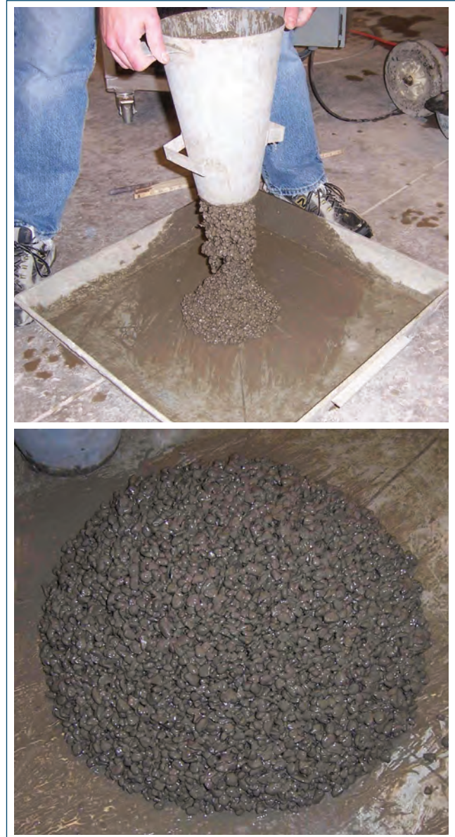
Figure 3-6. Fresh pervious concrete
