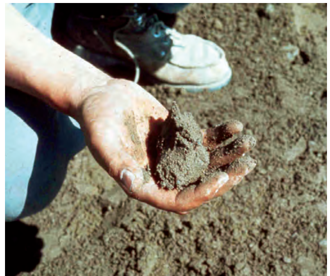
Figure 5-6. RCC material looks drier than conventional concrete
